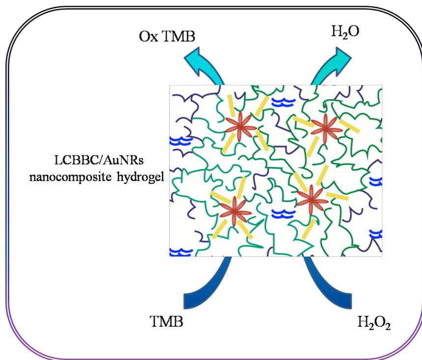
**Figure S5.** A schematic for catalytic activity based on LCBBC/AuNRs nanocomposite hydrogel in which LCBBC/AuNRs was used as peroxidase mimics to catalyze oxidation of peroxidase substrate 3,3,5,5-tetramethylbenzidine (TMB) in the presence of H<sub>2</sub>O<sub>2</sub> as oxidized
