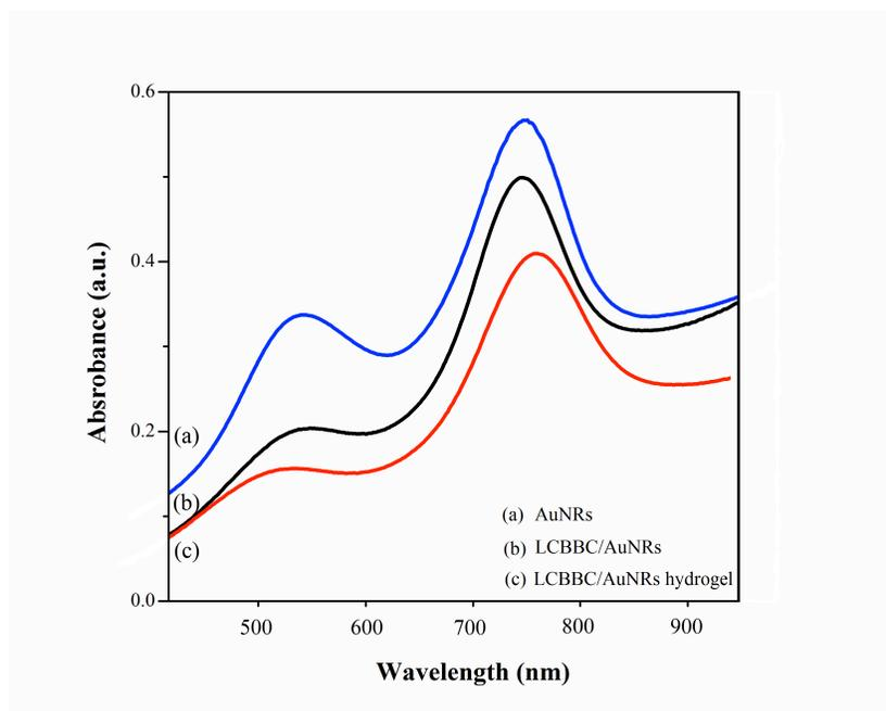
**Figure S1.** UV-visible absorption spectra of AuNRs, LCBBC/AuNRs in DMF solution, and LCBBC/AuNRs nanocomposite hydrogel. The absorbance of these samples exhibited two plasmon bands including shorter wavelength (transverse plasmon oscillation) at 520 nm and longer wavelength (longitudinal plasmon oscillation- LSPR) at 740 nm
