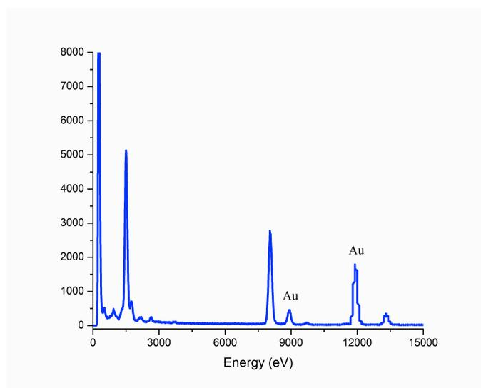
**Figure S3:** EDX spectroscopy of LCBBC/AuNRs nanocomposite hydrogel with a quantitative elemental composition of Au atom about 3.78 wt %
