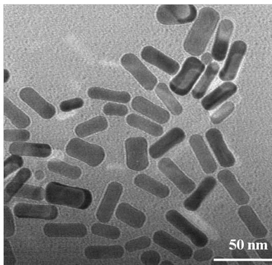
**Figure S2.** TEM image of ligand protected AuNRs by seed-mediated method with an average dimension of 25 x 5 nm, obtained by dropping solution of the nanorods on to copper grid coat with Formvar film, followed by air-drying
