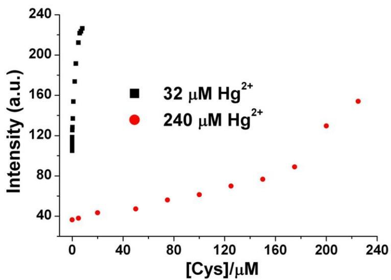
**Figure S6.** Fluorescence emission intensity (545 nm) of GE-Tb-DPA containing 32 μM or 240 μM Hg<sup>2+</sup> with increasing amounts of cysteine.
