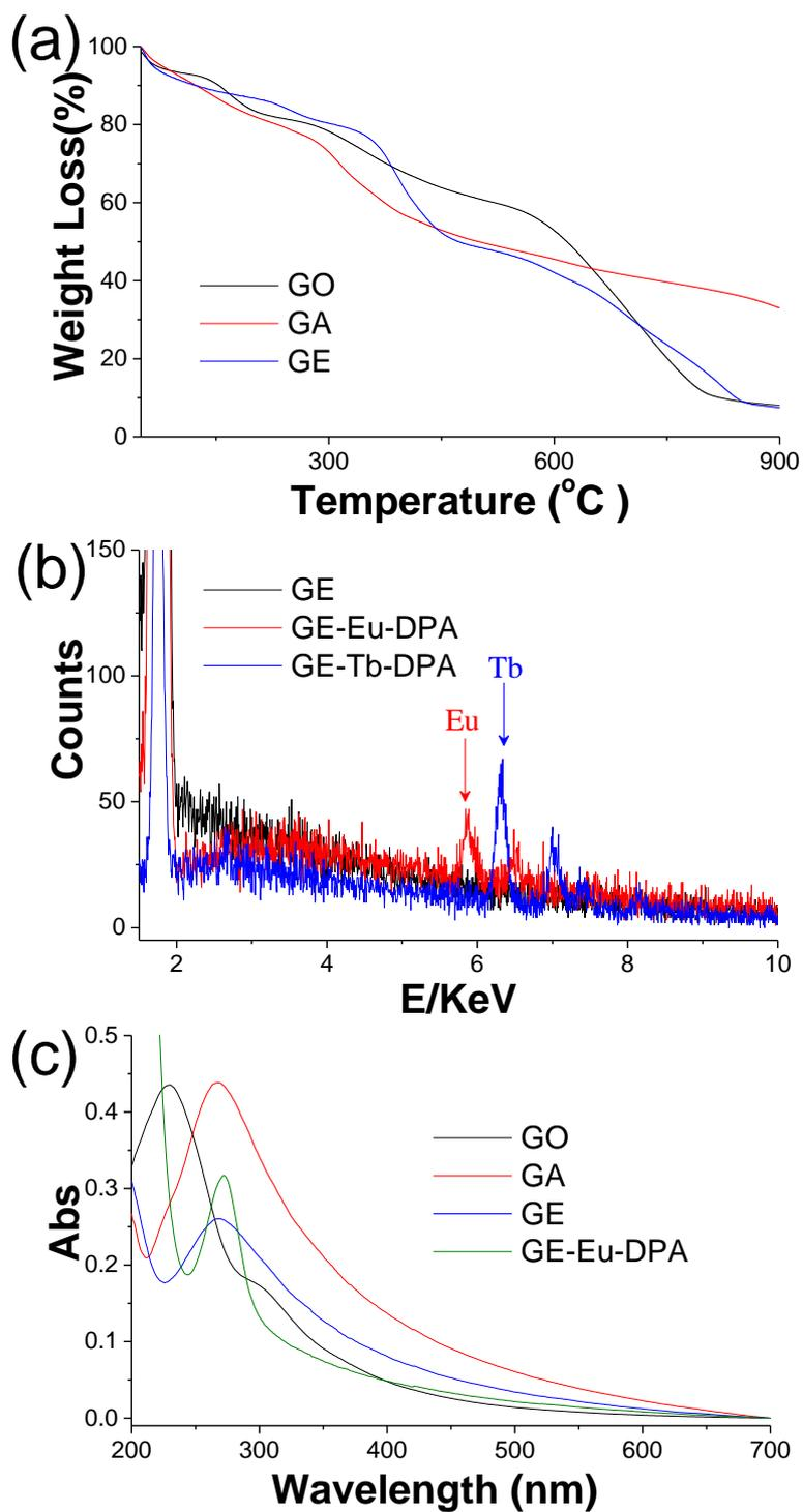
**Figure S3.** (a) Thermogravimetric analysis for GO (black), GA (red) and GE(blue) in  $N_2$  atmosphere with a ramp of  $10\text{ }^\circ\text{C}/\text{min}$ . (b) EDX spectra of GE (black), GE-Eu-DPA (red) and GE-Tb-DPA (blue). (c) UV/Vis spectra for GO (black), GA(red), GE(blue) and GE-Eu-DPA (green) in ddH<sub>2</sub>O.
