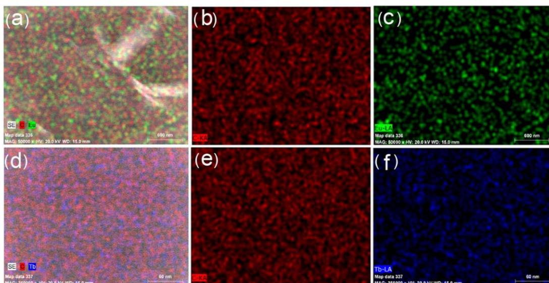
**Figure S4.** Elemental mapping images of GE-Eu-DPA or GE-Tb-DPA sheets. (a) the overlay of all the elemental mappings of GE-Eu-DPA, (b) Carbon and (c) Eu; (d) the overlay of all the elemental mappings of GE-Tb-DPA, (e) Carbon and (f) Tb. The images indicate the homogeneous dispersion of Eu and Tb on graphene sheets.
