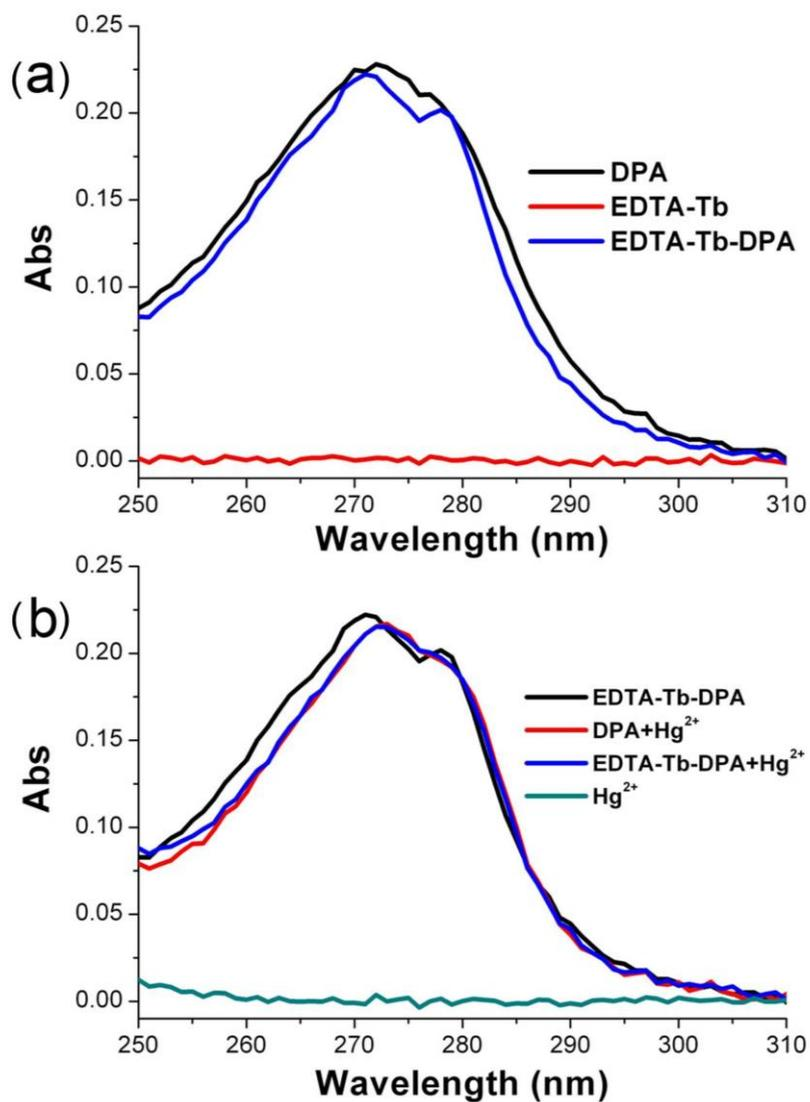
**Figure S5.** (a) UV/Vis spectra for 2.5 μM DPA (black), 2.5 μM EDTA-Tb (red) and 2.5 μM EDTA-Tb-DPA (blue) in ddH<sub>2</sub>O. (b) UV/Vis spectra for 2.5 μM EDTA-Tb-DPA (black), 2.5 μM DPA+ 50 μM Hg<sup>2+</sup> (red), 2.5 μM EDTA-Tb-DPA+ Hg<sup>2+</sup> (blue) and 50 μM Hg<sup>2+</sup> (cyan) in ddH<sub>2</sub>O.
