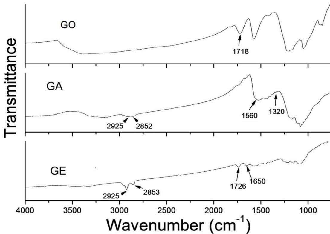
**Figure S2.** FT-IR spectra of GO, GA (Graphene-NH<sub>2</sub>) and GE (Graphene-EDTA).
