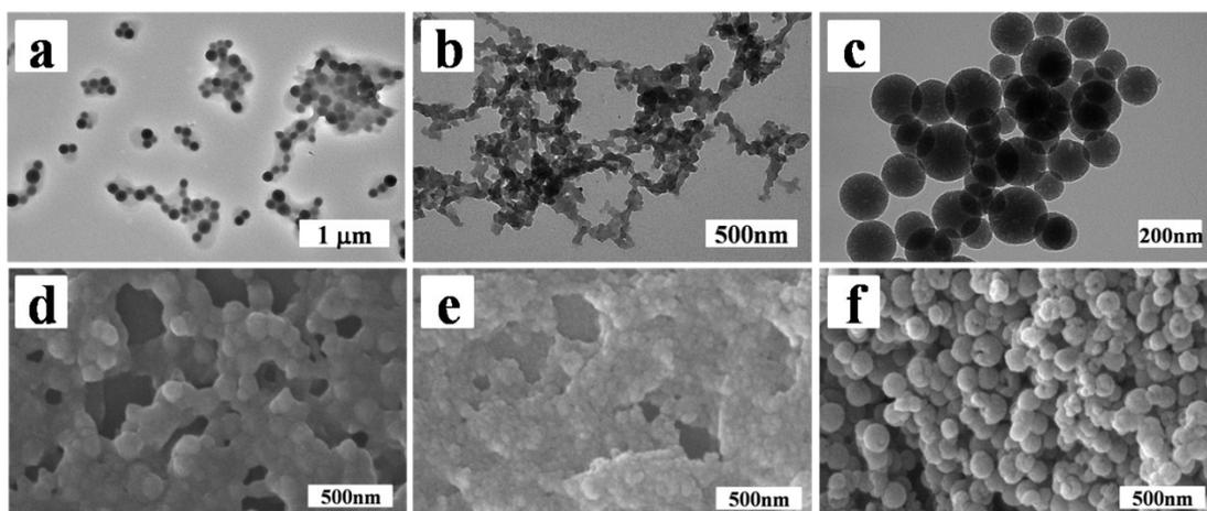
**Fig. S6** TEM images and FE-SEM images of resin/silica nanocomposites particles. Resin particles are obtained after etching silica and the resulted hollow silica particles are synthesized at 0.05 g of 3-aminophenol. a) TEM image and d) FE-SEM image of resin/silica nanocomposites particles. b) TEM image and e) FE-SEM image of resin particles after etching silica. c) TEM image and f) FE-SEM image of the resulted hollow silica particles.
