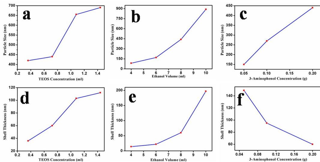
**Fig. S2** The hollow silica particle size and shell thickness as the function of TEOS concentration, ethanol volume and 3-aminophenol concentration. The detailed conditions can be seen in Table S1: (a and d) sample 1-4, (b and e) sample 2, 7, 8 and 9, (c and f) sample 2, 5 and 6.
