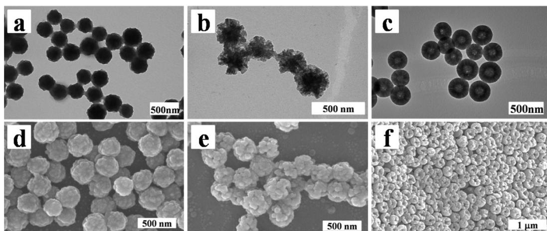
**Fig. S5** TEM images and FE-SEM images of resin/silica nanocomposites particles. Resin particles are obtained after etching silica and the resulted hollow silica particles are synthesized at 0.1 g of 3-aminophenol. a) TEM image and d) FE-SEM image of resin/silica nanocomposites particles. b) TEM image and e) FE-SEM image of resin particles after etching silica. c) TEM image and f) FE-SEM image of the resulted hollow silica particles.
