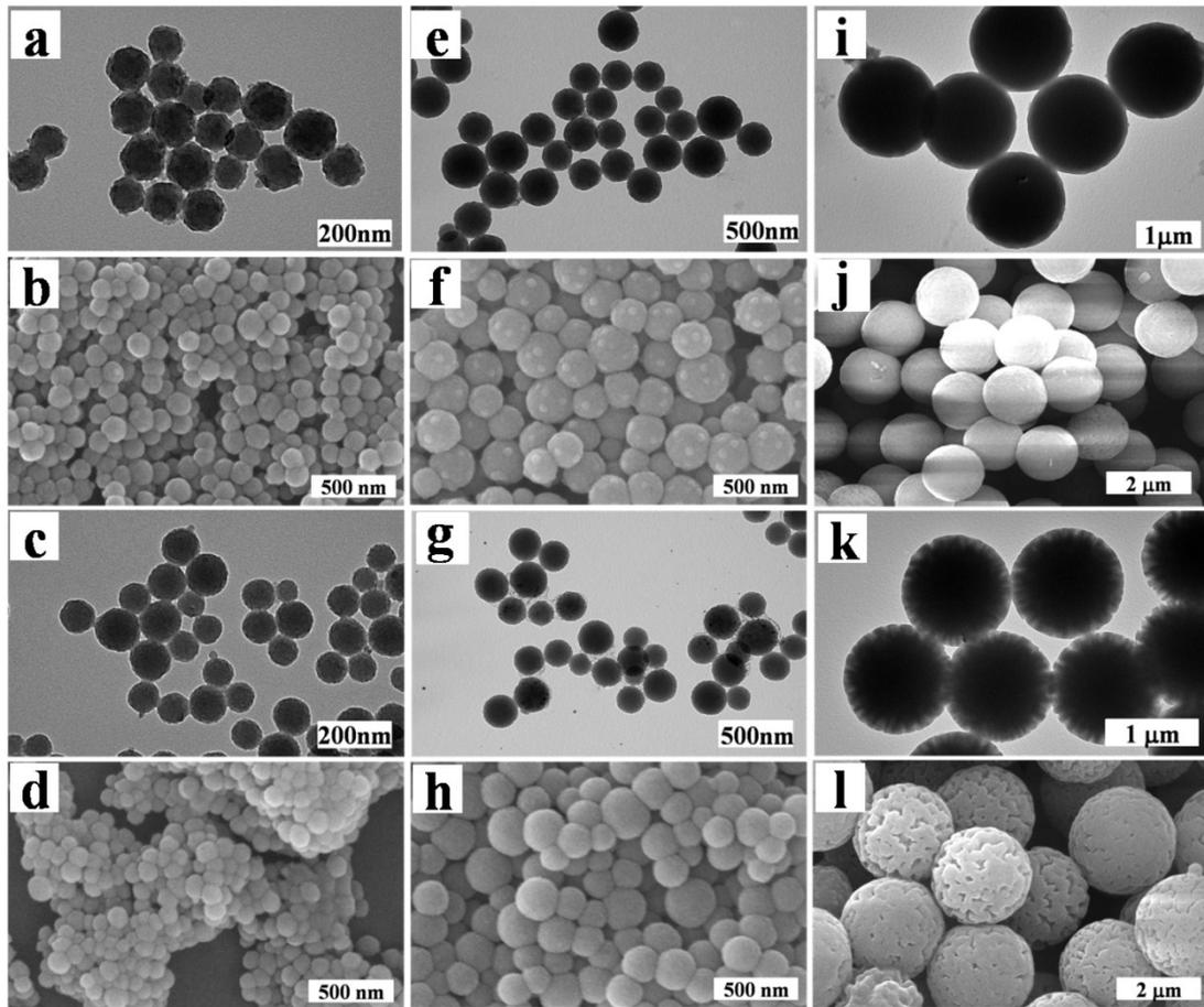
**Fig. S8** a, e and i) TEM images and b, f and j) FE-SEM images of resin/silica nanocomposites synthesized at 4 ml, 6 ml and 10 ml of ethanol, respectively. c, g and k) TEM images and d, h and l) FE-SEM images of the obtained resin particles after etching silica in the corresponding nanocomposite particles.
