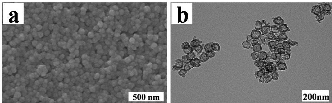
**Fig. S9** FE-SEM images (a) and TEM images (b) of hollow silica particles prepared at 4ml of ethanol.
