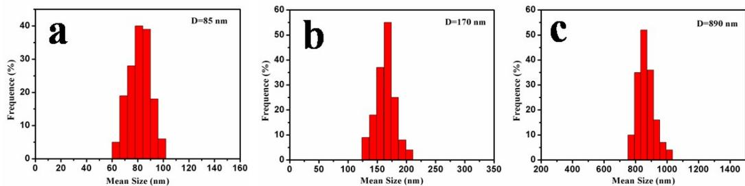
**Fig. S10** The size distribution of hollow silica particle obtained from more than 200 particles in the FE-SEM images. a) sample 7, b) sample 8, c) sample 9.
