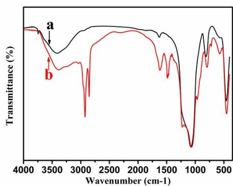
**Fig. S7** FT-IR spectra of a) the obtained particles after calcinating and b) as-synthesized resin/silica nanocomposites particles of sample 5. The characteristic peaks of aliphatics at 2850-2950  $\text{cm}^{-1}$  in resin disappear after calcinating(a), confirming the complete removal of resin.<sup>23</sup>
