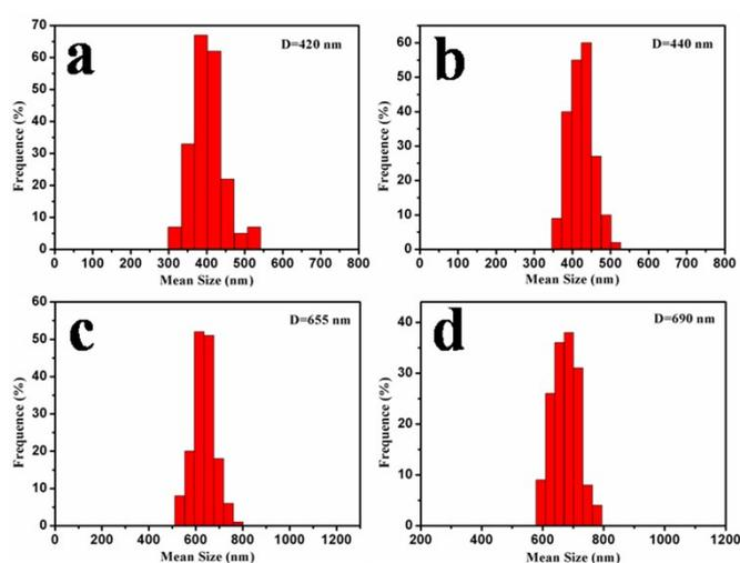
**Fig. S1** The hollow silica particle size distribution of a) sample 1, b) sample 2, c) sample 3 and d) sample 4, obtained from more than 200 particles in the FE-SEM images.
