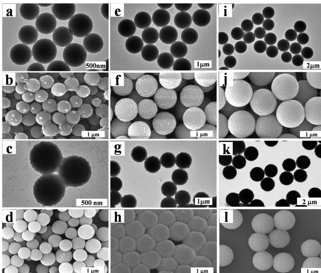
**Fig. S4** a, e and i) TEM images and b, f and j) FE-SEM images of resin/silica nanocomposites synthesized at 0.36 ml, 1.08 ml and 1.44 ml of TEOS, respectively. c, g and k) TEM images and d, h and l) FE-SEM images of the obtained resin particles after etching silica in the corresponding nanocomposite particles.
