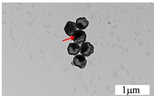
**Fig. S3** TEM image of NaCl-encapsulated hollow mesoporous silica particles. The red arrow shows the NaCl microcrystal located in the hollow particle.
