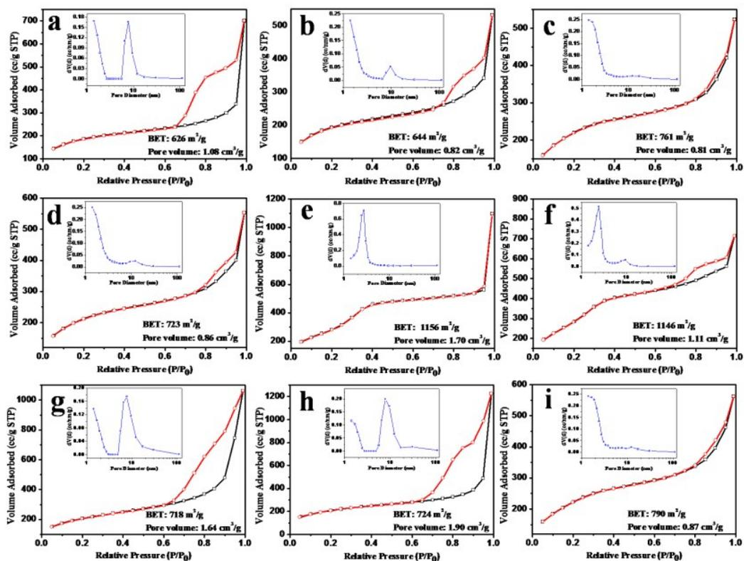
**Fig. S11** Nitrogen adsorption–desorption isotherms of a)-i) samples 1-9, respectively. The insets correspond to the pore size distribution curves.
