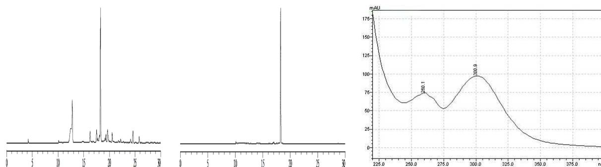
**Fig. S1** Reversed-phase HPLC traces for Pt-c(RGDfK) conjugate (3): reaction crude (left) and purified (center), and UV-Vis spectrum of the compound in ACN/H<sub>2</sub>O solvent (right).
