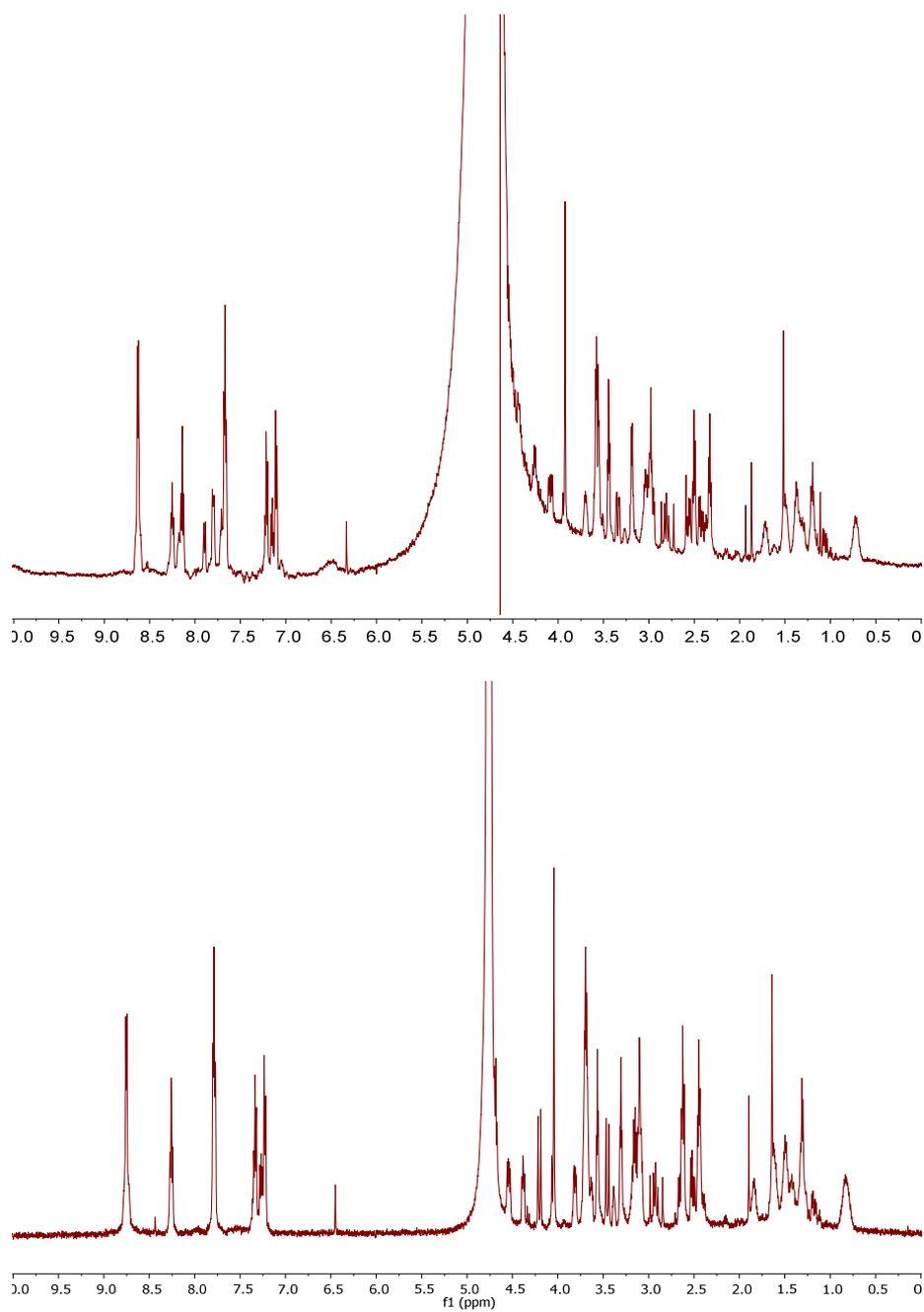
**Fig. S3.** 500 MHz <sup>1</sup>H NMR spectra of conjugate 3 in H<sub>2</sub>O/D<sub>2</sub>O 9:1 v/v (top) and in D<sub>2</sub>O (bottom).
