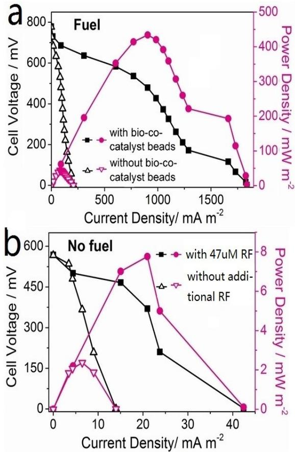
Fig. S3. Power output and polarization curves of MFCs (a) with fuel using carbon cloth anodes without oxygen plasma treatment. RF concentration in MFC anodic chamber containing bio-cocatalyst beads accumulated to  $46.84 \pm 0.24 \mu\text{M}$  ( $n=3$ ) after loading these beads for about 66h. (b) without fuel.  $47 \mu\text{M}$  RF was added into the MFC anodic chamber containing anolyte without lactate.
