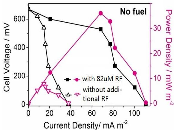
Fig. S2. Power output and polarization curves of MFCs without fuel using oxygen plasma treated carbon cloth anodes. 82 μM RF was added into the MFC anodic chamber containing anolyte without lactate.
