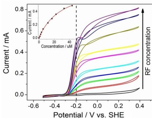
Fig. S4. Typical cyclic voltammograms (1 mV/s) from a *S. oneidensis* MR-1 biofilm residing on anodic carbon cloth without O<sub>2</sub> plasma treatment in 0, 1.1, 2.16, 3.22, 5.34, 11.8, 17, 22.3, 32.9 and 43.5 μM RF. The electrochemical potential (-0.2 V) where catalytic current was analyzed is illustrated by a dash line. Inset: Variation of the magnitude of the catalytic current, measured at -
