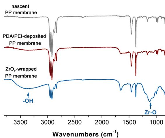
**Figure S3** FT-IR/ATR spectra of the nascent, PDA/PEI-deposited and ZrO<sub>2</sub>-wrapped polypropylene membranes.
