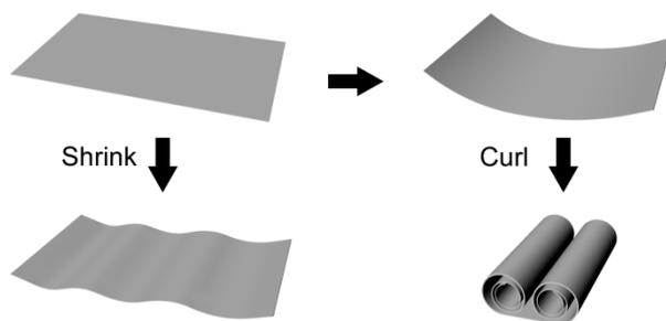
**Figure S1** Schematic representation of shrinkage and curling for polymer membranes.
