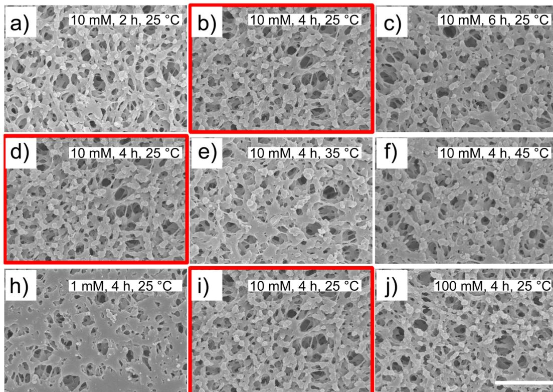
**Figure S2** SEM images of ZrO<sub>2</sub>-wrapped polypropylene membranes fabricated with different hydrolysis time, temperature and HCl concentration. The scale bar is 1  $\mu$ m.
