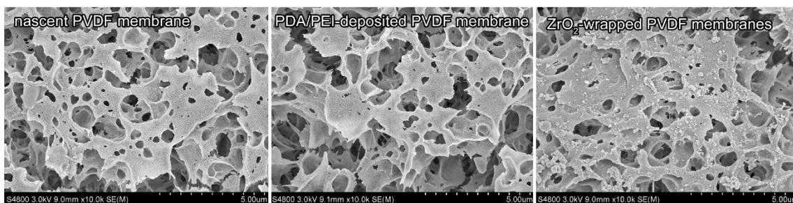
**Figure S6** SEM images of the nascent, PDA/PEI-deposited and ZrO<sub>2</sub>-wrapped PVDF membranes.
