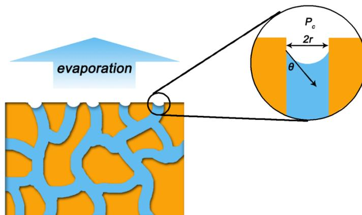
**Figure S5** Schematic representation of the internal pressure in hydrophilic pores.
