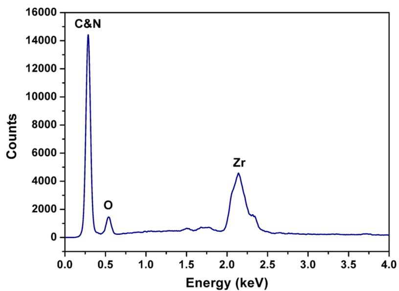
**Figure S4** Typical EDX spectrum from the cross-section of a  $\text{ZrO}_2$ -wrapped membrane.
