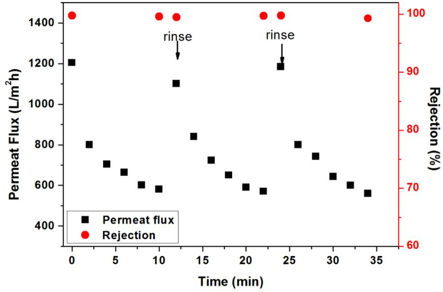
**Figure 9** The flux recovery of ZrO<sub>2</sub>-wrapped membranes during the diesel-in-water emulsion filtration.
