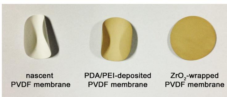
**Figure S7** Digital photograph of the nascent, PDA/PEI-deposited and ZrO<sub>2</sub>-wrapped PVDF membranes after thermal treated at 120 °C for 1 h.
