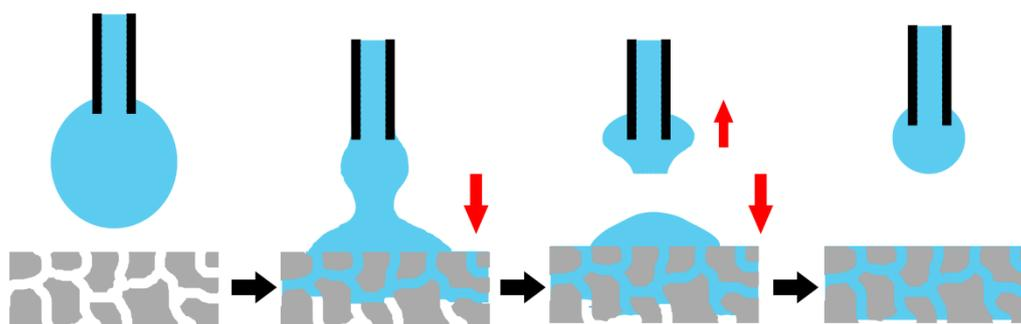
**Figure S8** Schematic representation for breakup of a water drop when it contacts a hydrophilic porous substrate.
