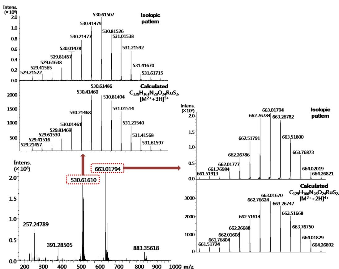
**Fig. S1.** The HR-ESI-MS spectra of Ru-SST **8** (calcd exact mass: 530.61486  $[M^{2+}+3H]^{5+}$ , 663.01670  $[M^{2+}+2H]^{4+}$ , formula:  $C_{129}H_{158}N_{28}O_{24}RuS_2$ ).
