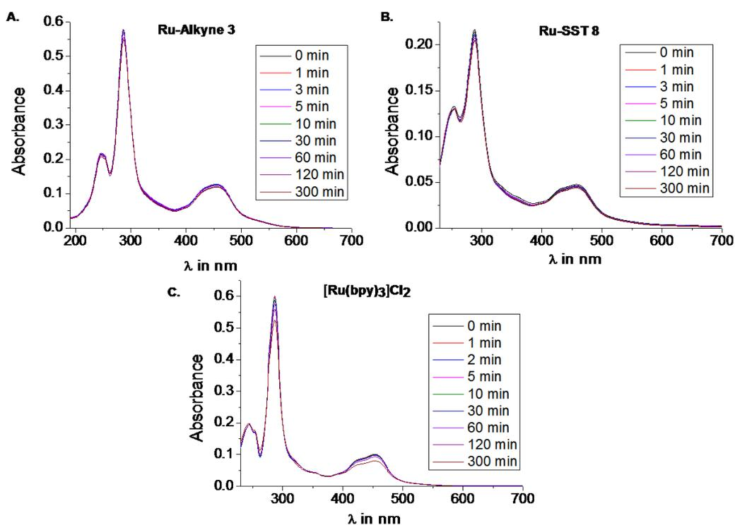
**Fig. S3.** Photostability of Ru-Alkyne **3** (A), Ru-SST **8** (B) and a typical ruthenium(II) polypyridine [Ru(bpy)<sub>3</sub>]Cl<sub>2</sub> (C) in MilliQ water ( $c = 1 \times 10^{-5}$  mol/L).
