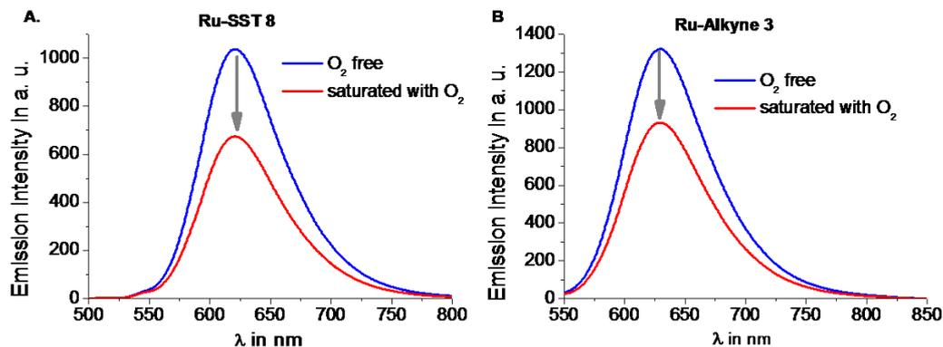
**Fig. S4.** Emission spectra ( $\lambda_{\text{ex}} = 460 \text{ nm}$ ,  $c = 1 \times 10^{-5} \text{ mol/L}$ ) of Ru-SST **8** (A) and Ru-Alkyne **3** (B) in MilliQ water saturated with O<sub>2</sub> (red) and O<sub>2</sub> free (blue).
