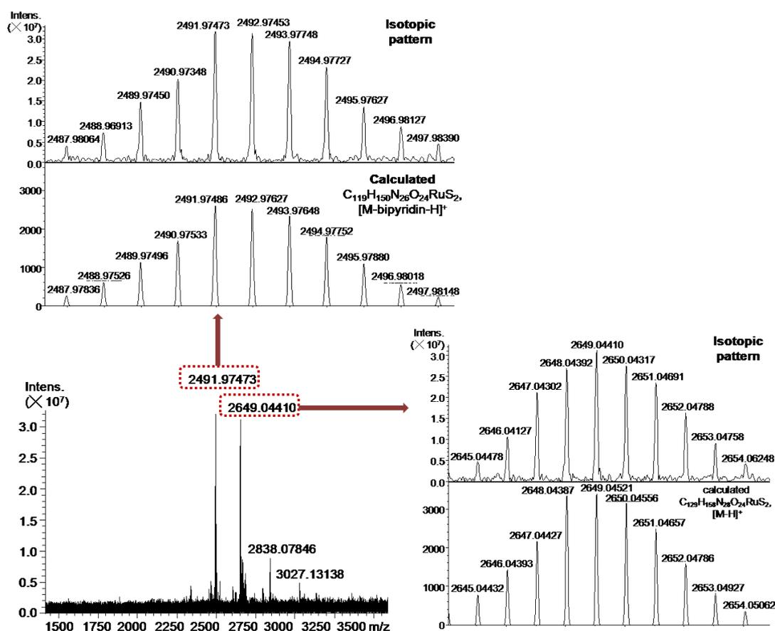
**Fig. S2.** The HR-MALDI-MS spectra of Ru-SST **8** with  $\alpha$ -cyano-4-hydroxycinnamic acid as matrix (calcd exact mass: 2491.97486 [M-bipyridin-H]<sup>+</sup>, 2649.04521 [M-H]<sup>+</sup>, formula: C<sub>129</sub>H<sub>158</sub>N<sub>28</sub>O<sub>24</sub>RuS<sub>2</sub>).
