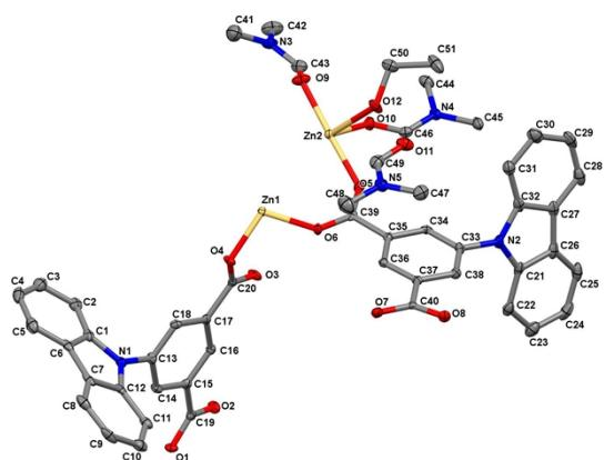
**Figure S11.** ORTEP of ZnCbz MOF asymmetric unit (generated by Mercury).
