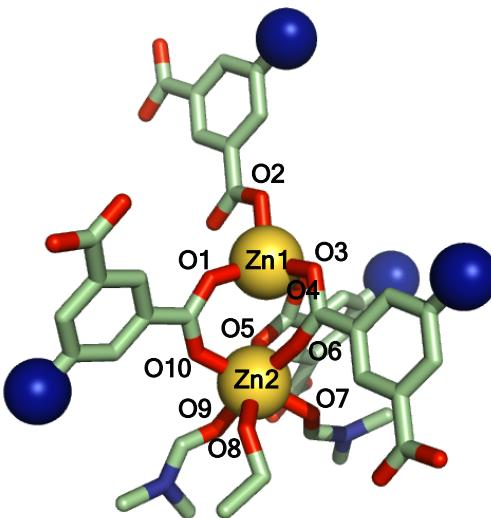
**Figure S14.** Secondary-building unit (SBU) in ZnCbz MOF. Carbon = pale green; oxygen = red; nitrogen = blue; zinc = yellow. Carbazoles as blue spheres
