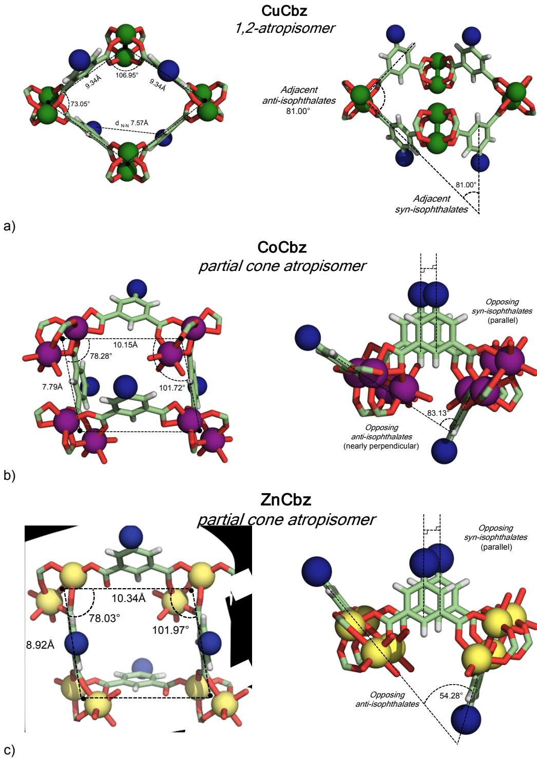
**Figure S15.** Left: Bonds and angles of parallelograms formed by SBUs centroids in Cbz MOF structures. Right: Dihedral angles between isophthalates of one square unit of the square grids of Cbz MOFs. Carbon = pale green; oxygen = red; copper = green; cobalt = purple; zinc = yellow; carbazoles = blue spheres.
