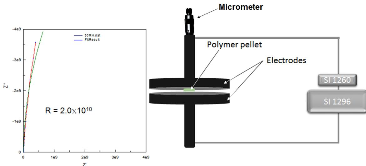
**Fig. S4.** Nyquist plot for impedance measurement at very low humidity for **polyMo** and the schematic of the conductivity measurement setup.
