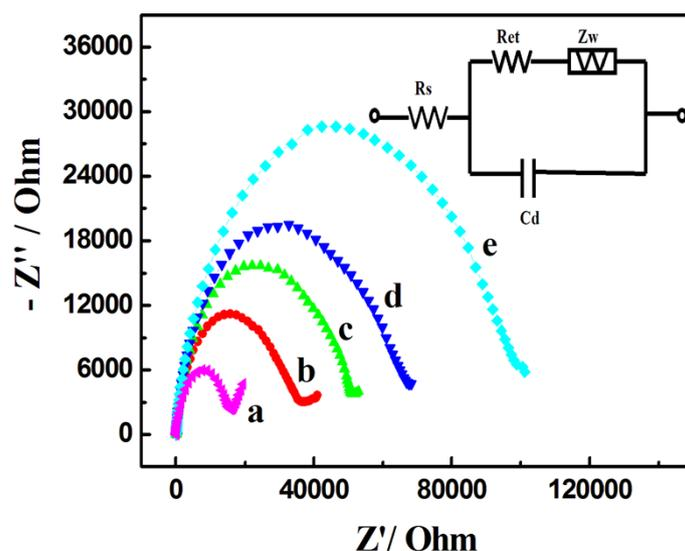
**Fig. S1** The Nyquist plots obtained for electrode which was immobilized by Ab<sub>1</sub> (a), Ab<sub>1</sub>/PSA (b), Ab<sub>1</sub>/PSA/Ab<sub>2</sub> (c), Ab<sub>1</sub>/PSA/Ab<sub>2</sub>/streptavidin (d), Ab<sub>1</sub>/PSA/Ab<sub>2</sub>/streptavidin/biotin-Nb.BtSI (e) in 5 mM [Fe(CN)<sub>6</sub><sup>3-/4-</sup>] and 0.1M KCl solution.
