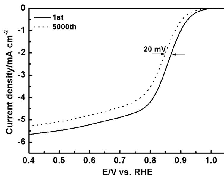
**Figure S13.** Linear scan voltammograms (LSVs) of the (Fe, Co)@NGC NCs in O<sub>2</sub>-saturated 0.1 M KOH at a scan rate of 5 mV s<sup>-1</sup> and a rotating rate of 2400 rpm.
