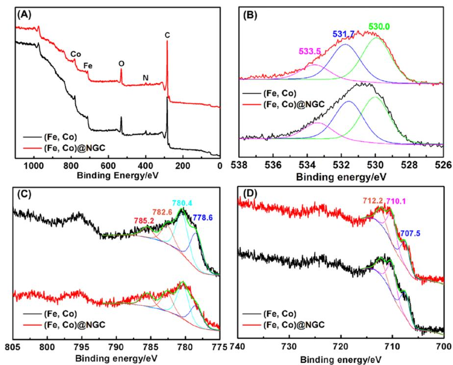
**Figure S8.** (A) The XPS full spectra, (B) O 1s, (C) Co 2p, and (D) Fe 2p XPS spectra of the (Fe, Co) and (Fe, Co)@NGC NCs.
