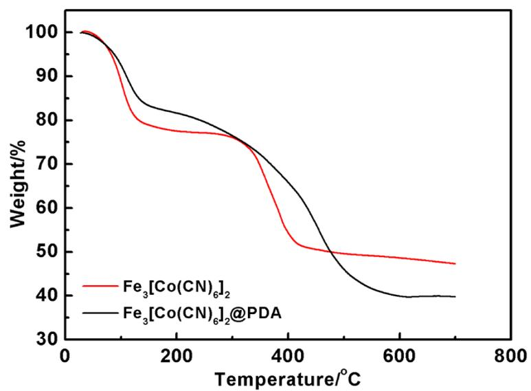
**Figure S4.** TGA curves of the  $\text{Fe}_3[\text{Co}(\text{CN})_6]_2$  and  $\text{Fe}_3[\text{Co}(\text{CN})_6]_2@\text{PDA}$  NCs under Ar atmosphere in the temperature range of 30 ~ 700 °C with a heating rate of 10 °C min<sup>-1</sup>.
