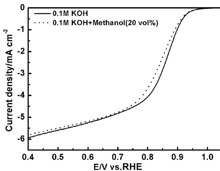
**Figure S12.** Linear scan voltammograms (LSVs) of the (Fe, Co)@NGC NCs in O<sub>2</sub>-saturated 0.1M KOH and 0.1 M KOH (20 vol% of methanol) at a scan rate of 5 mV s<sup>-1</sup> and a rotating rate of 2400 rpm.
