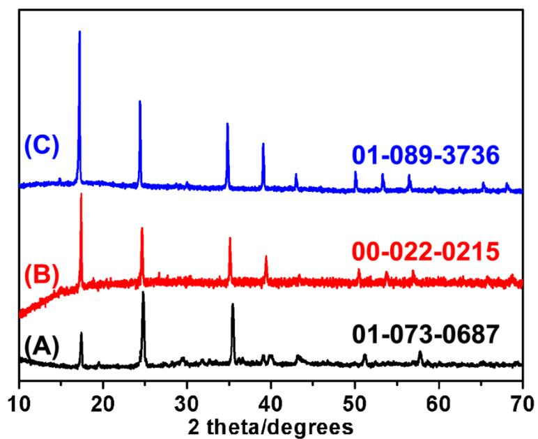
**Figure S2.** XRD patterns of (A)  $\text{Fe}_4[\text{Fe}(\text{CN})_3]_2$ , (B)  $\text{Co}_3[\text{Co}(\text{CN})_6]_2$ , and (C)  $\text{Fe}_3[\text{Co}(\text{CN})_6]_2$  precursors, which are in agreement with the standard patterns of JCPDS 01-073-0687, 00-022-0215, and 01-089-3736, respectively.
