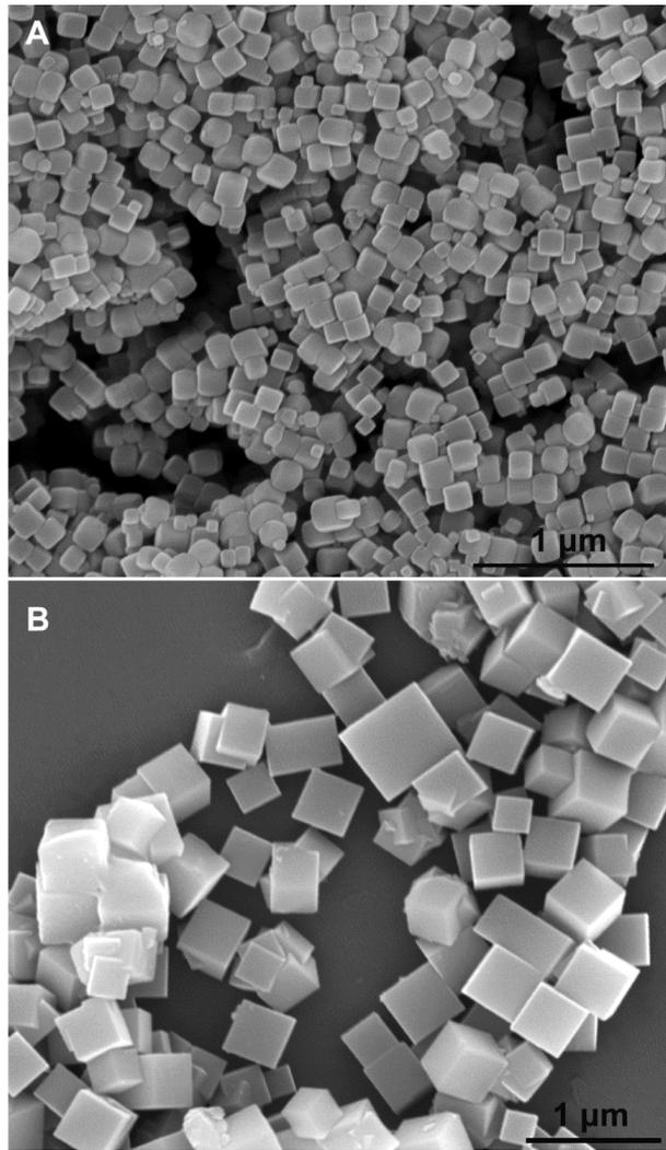
**Figure S1.** SEM images of (A)  $\text{Co}_3[\text{Co}(\text{CN})_6]_2$  and (B)  $\text{Fe}_3[\text{Fe}(\text{CN})_6]_2$  precursors.
