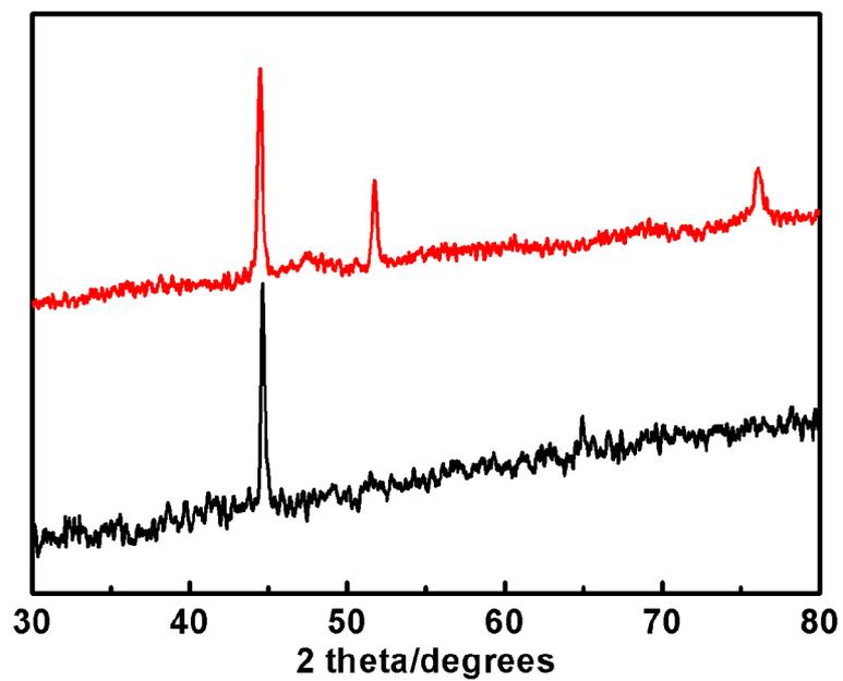
**Figure S7.** XRD patterns of the products derived from  $\text{Fe}_3[\text{Fe}(\text{CN})_6]_2$  (black) and  $\text{Co}_3[\text{Co}(\text{CN})_6]_2$  (Red) at 700 °C for 1 h under Ar atmosphere.
