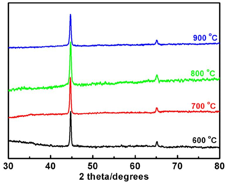
**Figure S3.** XRD patterns of the products transformed from  $\text{Fe}_3[\text{Co}(\text{CN})_6]_2$  NCs at 600-900 °C under Ar atmospheres.
