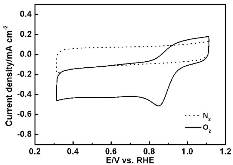
**Figure S9.** CV curves of the (Fe, Co) NCs in N<sub>2</sub>-saturated (dash line) or O<sub>2</sub>-saturated (solid line)
