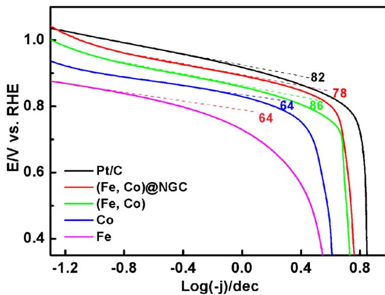
**Figure S11.** The Tafel plots of the Pt/C, (Fe, Co)@NGC, (Fe, Co), Co, and Fe catalysts measured in O<sub>2</sub>-saturated 0.1 M KOH aqueous solution at 2400 rpm.
