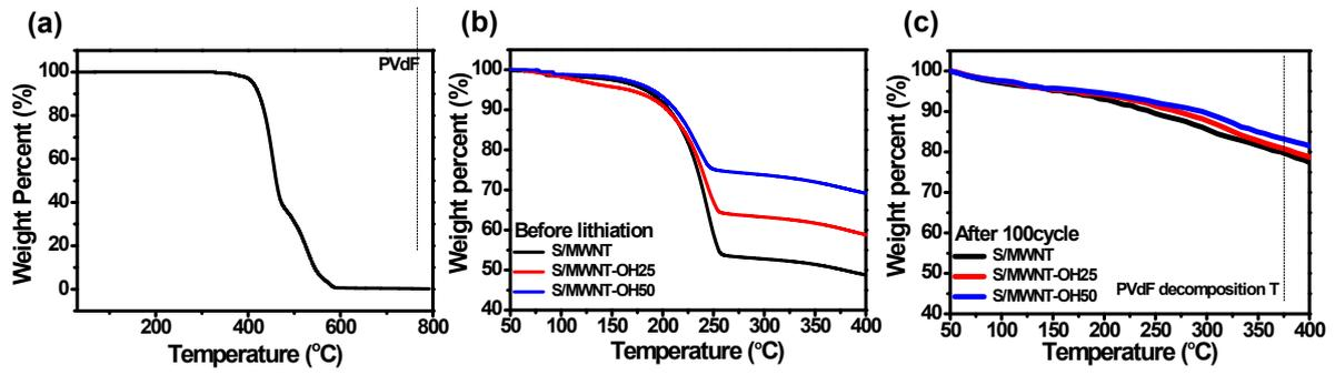
Figure S4. TGA curves of (a) PVdF and (b) before, (c) after 100 cycles of each S/MWNT, S/MWNT-OH25, and S/MWNT-OH50 electrodes
