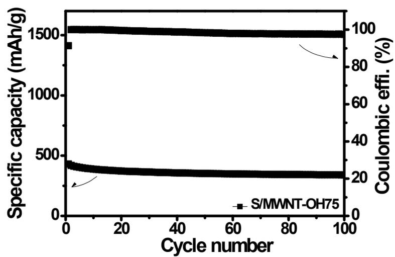
Figure S6. Cycle performance and Coulombic efficiency of S/MWNT-OH75 electrode during 100 cycles
