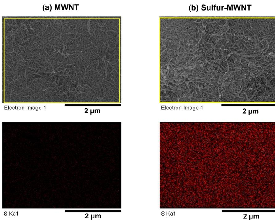
Figure S1. SEM EDS analysis of MWNT and Sulfur-MWNT.
