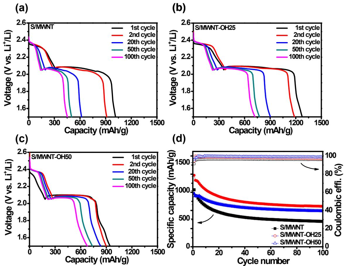
Figure S3. Discharge profiles of (a) S/MWNT, (b) S/MWNT-OH25, (c) S/MWNT-OH50. (d) Cycle performance of each electrodes at 0.2C
