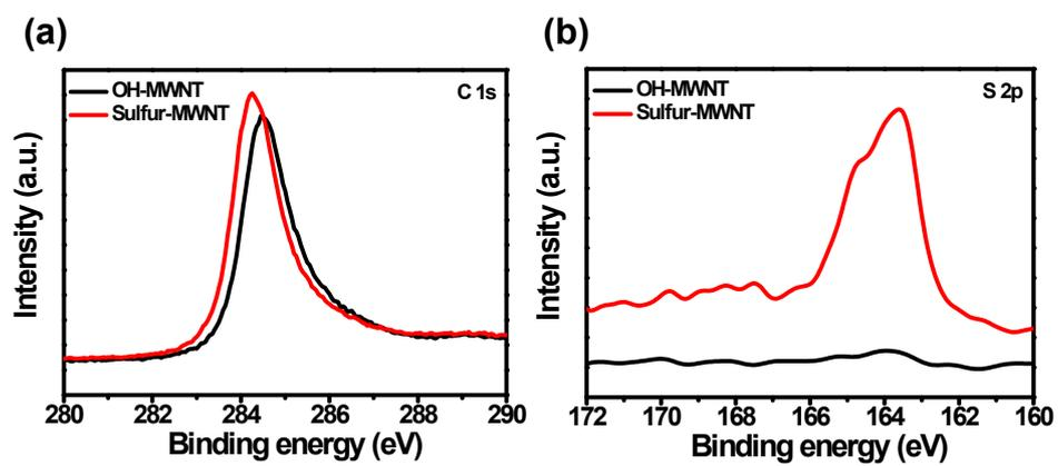
Figure S2. (a) C 1s XPS spectra of OH-MWNT and Sulfur-MWNT, (b) S 2p XPS spectra of OH-MWNT
