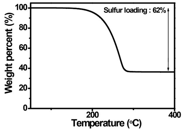
Figure S5. TGA curves of Sulfur-MWNT composite
