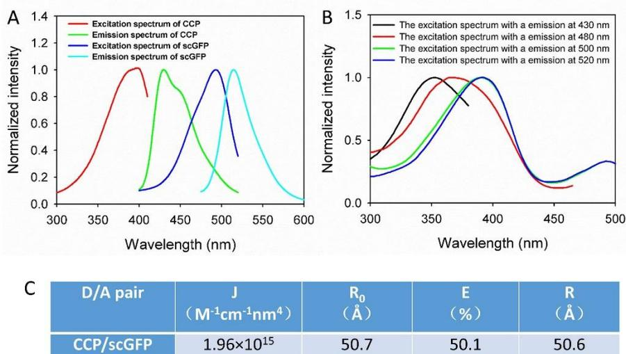
Figure S1. (A) The excitation and emission spectra of CCP and scGFP, respectively. (B) Excitation spectra of scGFP/poly(ADP-ribose)ated PARP-1/CCP complex monitored at different emission wavelengths. (C) The data summary of spectra overlap integral (J), Förster distance ( $R_0$ ), energy transfer efficiency (E) and donor-acceptor distance (R).
