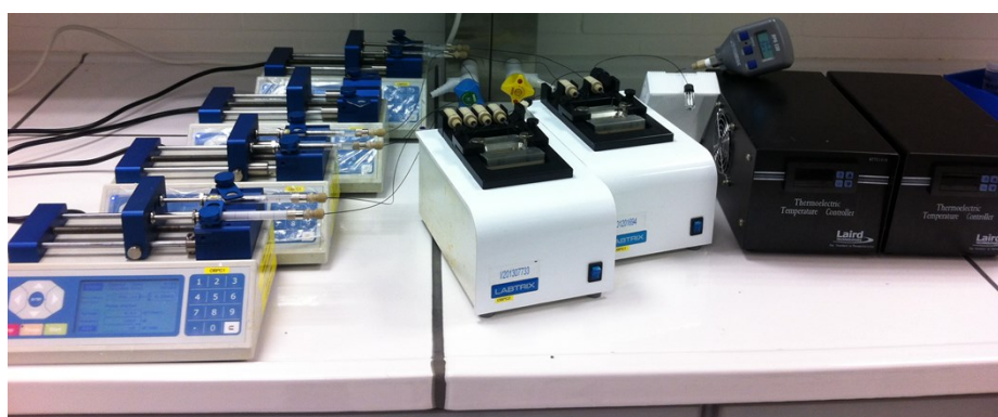
Figure S1: Microreactor cascade set-up as used for the triblock copolymerizations.
