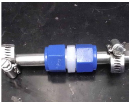
Figure S1: Picture of a Swagelok cell setup used for electrochemical testing.
