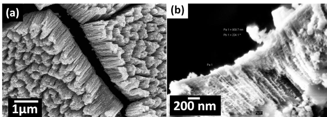
Figure S1: FESEM cross-sectional images of the fabricated (a) thick-walled and (b) thin-walled nanotubes
