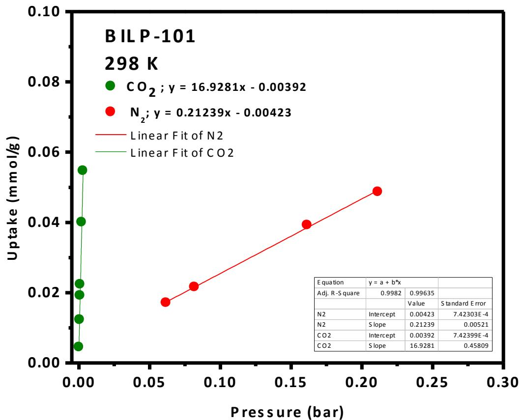
**Figure S11:** Experimental data (symbol) and corresponding fittings (solid line) of CO<sub>2</sub> (A) and N<sub>2</sub> (B) adsorption isotherms in BILP-101 at 298 K.
