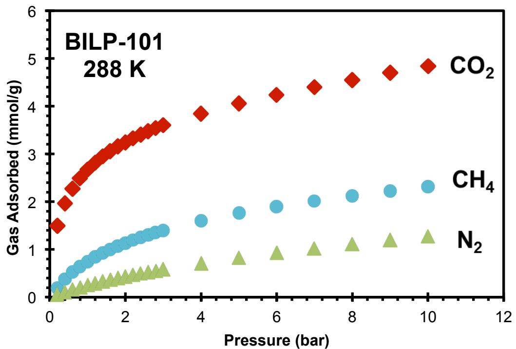
**Figure S8b:** CO<sub>2</sub> (Red diamond), CH<sub>4</sub> (Blue circle) and N<sub>2</sub> (Green triangle) uptake isotherms collected at 0.2-10 bar and 298 K using gravimetric sorption analysis.
