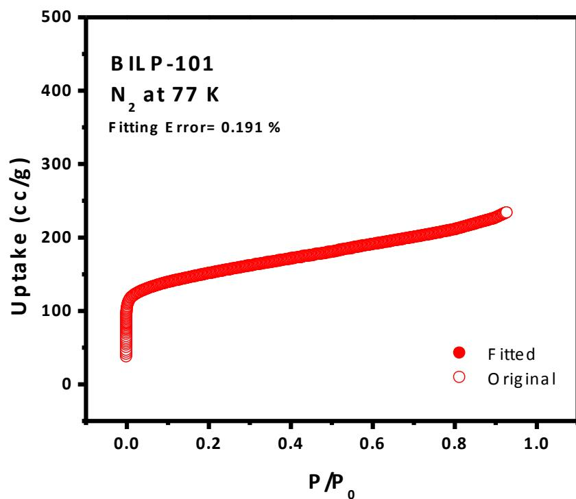
**Figure S6:** BET plot for BILP-101 calculated from the N<sub>2</sub> isotherm at 77K.
