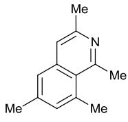
Flash column chromatography on a silica gel (ethyl acetate: petroleum ether, 1: 50) give **3da** (24.5 mg, 33% yield) as yellow oil.
