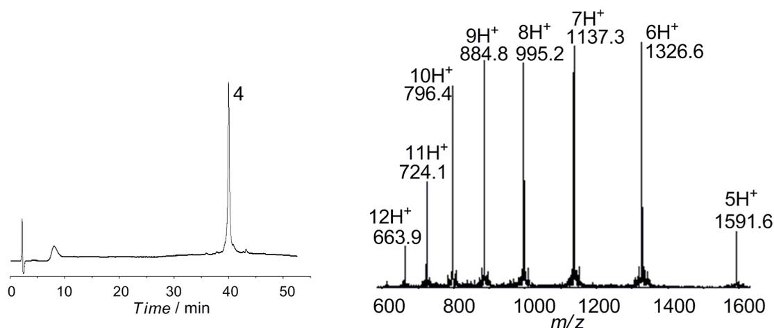
**Figure S27.** Characterization of **4**, the ligation product of **1** with **2**, by analytical RP-HPLC chromatogram ( $\lambda = 214$  nm) and ESI-MS. HPLC conditions: a linear gradient of 20-60% acetonitrile (with 0.08-0.1% TFA) in water (with 0.1% TFA) over 50 min (5% for 2 min, then 20% for 20 min, then 20%-60% for 30 min) on a Vydac C8 ( $4.6 \times 150$  mm) column. The ESI-MS spectrum gave an observed mass of 7954.2 Da (calcd 7955.2 Da, average isotopes).
