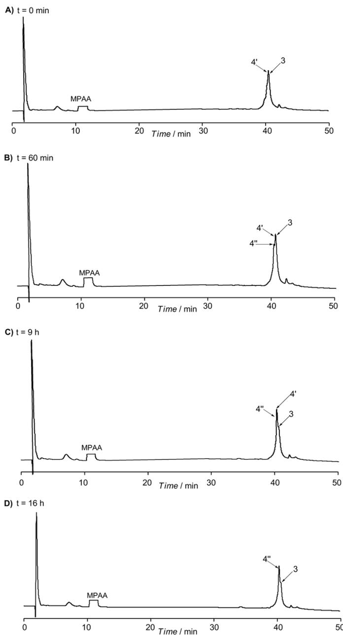
**Figure S22.** The failed ligation reaction between peptide hydrazide **4** (8.0 mg, 1  $\mu\text{mol}$ , 1 equiv.) and peptide amide **3** (4.6 mg, 1.5  $\mu\text{mol}$ , 1.5 equiv.). The major procedures were the same as described
