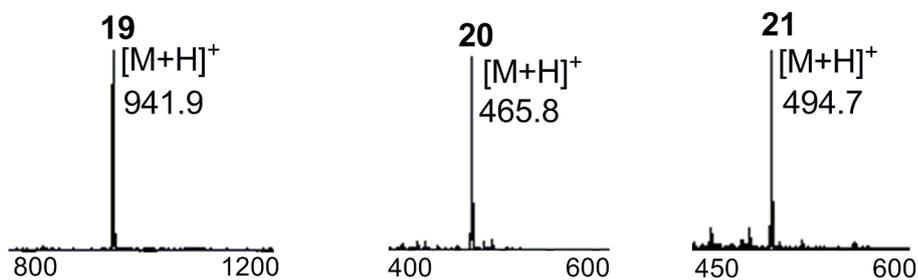
**Figure S32.** The ESI-MS spectra of purified **19**, **20** and **21**. For **19**, observed mass = 940.9 Da (calcd 940.1 Da, average isotopes). For **20**, observed mass = 464.8 Da (calcd 464.6 Da, average isotopes). For **21**, observed mass = 493.7 Da (calcd 493.5 Da, average isotopes).
