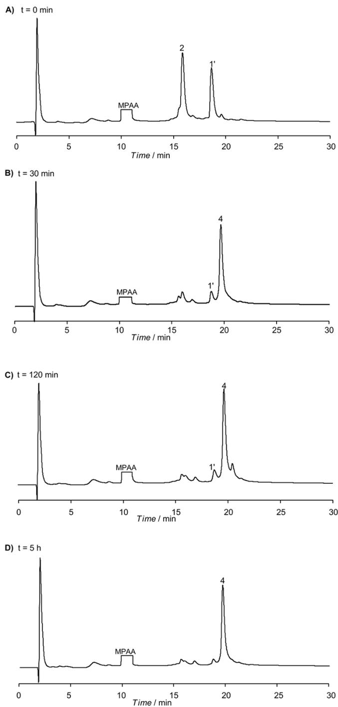
**Figure S21.** The ligation reaction between peptide hydrazide **1** and peptide hydrazide **2**. The ligation was monitored by analytical RP-HPLC chromatograms ( $\lambda = 214$  nm). Time points: 0 min, 30 min, 120 min and 5 h after the addition of peptide hydrazide **2**. The peak marked with **1'** corresponds to the peptide thioester generated from peptide hydrazide **1**. HPLC conditions: a linear gradient of 20-
