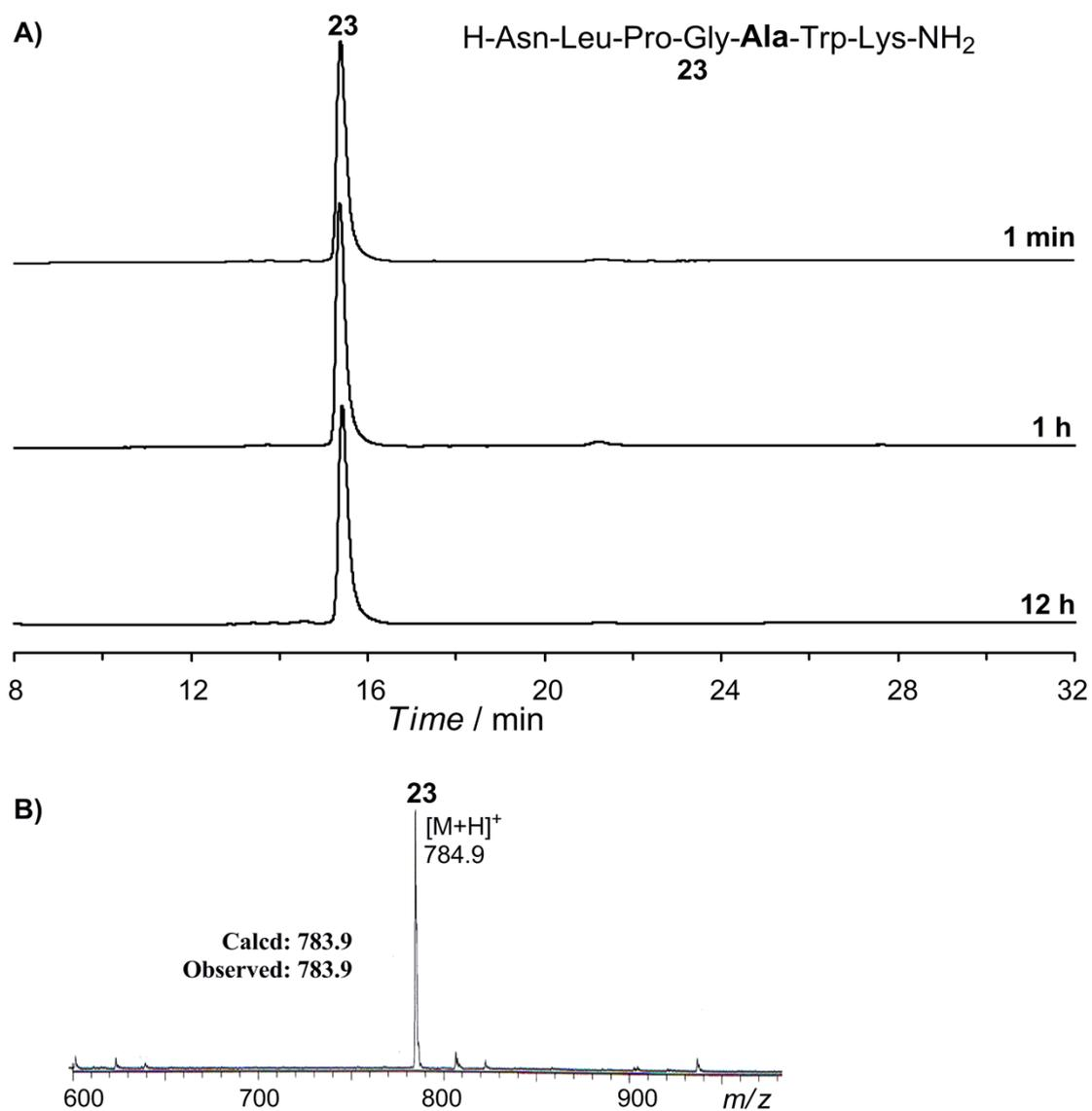
**Figure S16.** A) The reaction mixture of **23** was monitored by analytical RP-HPLC chromatograms ( $\lambda = 214$  nm). HPLC conditions: a linear gradient of 5-50% acetonitrile (with 0.08-0.1% TFA) in water (with 0.1% TFA) over 30 min (5% for 2 min, then 5%-50% for 30 min) on a Vydac C18 (4.6  $\times$  150 mm) column. B) The ESI-MS spectrum of purified **23**.
