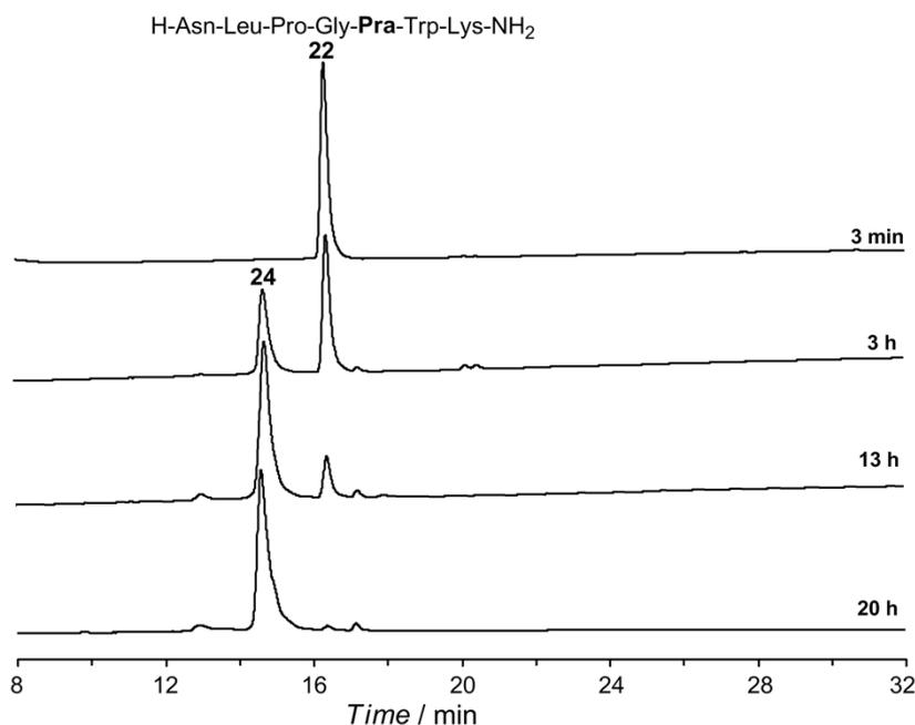
**Figure S17.** The reaction mixture of **22** was monitored by analytical RP-HPLC chromatograms ( $\lambda = 214$  nm). HPLC conditions: a linear gradient of 5-50% acetonitrile (with 0.08-0.1% TFA) in water (with 0.1% TFA) over 30 min (5% for 2 min, then 5%-50% for 30 min) on a Vydac C18 (4.6  $\times$  150 mm) column.
