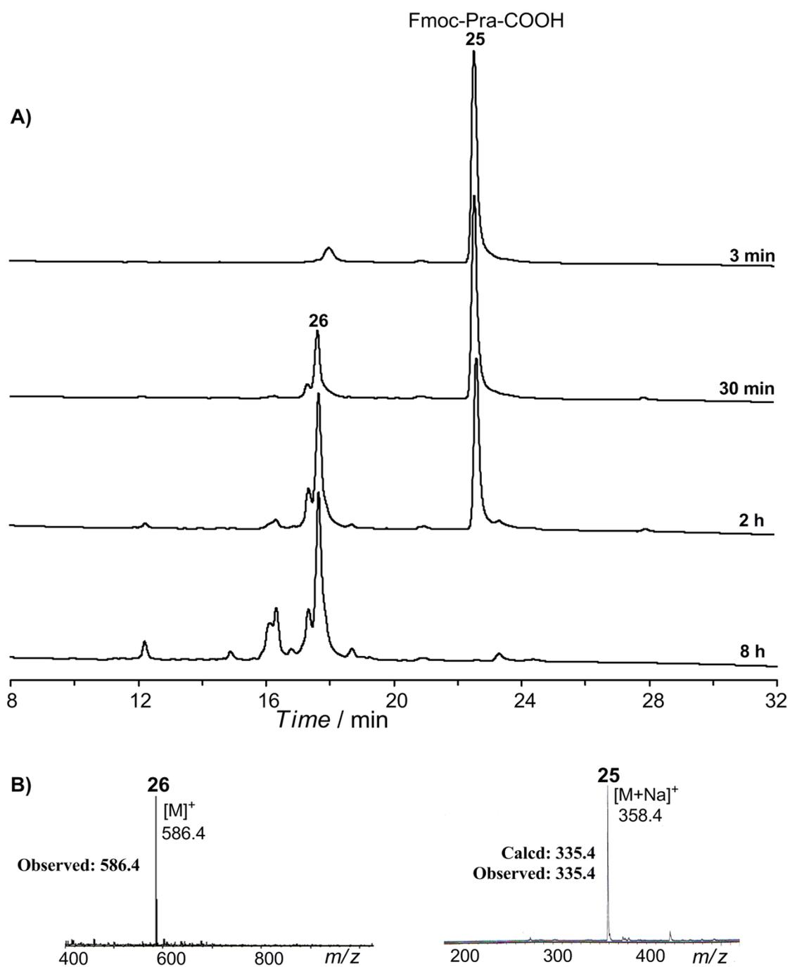
**Figure S14.** A) The reaction mixture of **25** were monitored by analytical RP-HPLC chromatograms ( $\lambda = 214$  nm). HPLC conditions: a linear gradient of 5-80% acetonitrile (with 0.08-0.1% TFA) in water (with 0.1% TFA) over 30 min (5% for 2 min, then 5%-80% for 30 min) on a Vydac C18 (4.6  $\times$  150 mm) column. B) The ESI-MS spectra of purified **25** and **26**.
