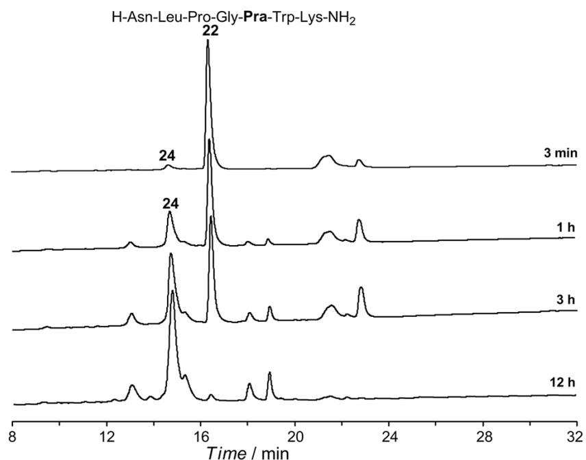
**Figure S19.** The reaction mixture of **22** was monitored by analytical RP-HPLC chromatograms ( $\lambda = 214$  nm). HPLC conditions: a linear gradient of 5-50% acetonitrile (with 0.08-0.1% TFA) in water (with 0.1% TFA) over 30 min (5% for 2 min, then 5%-50% for 30 min) on a Vydac C18 (4.6  $\times$  150 mm) column.
