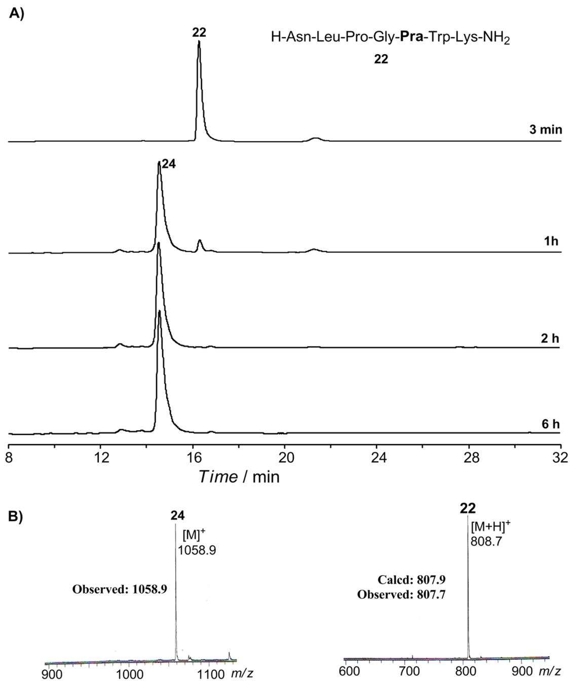
**Figure S15.** A) The reaction mixture of **22** was monitored by analytical RP-HPLC chromatograms ( $\lambda = 214$  nm). HPLC conditions: a linear gradient of 5-50% acetonitrile (with 0.08-0.1% TFA) in water (with 0.1% TFA) over 30 min (5% for 2 min, then 5%-50% for 30 min) on a Vydac C18 (4.6  $\times$  150 mm) column. B) The ESI-MS spectra of purified **24** and **22**.
