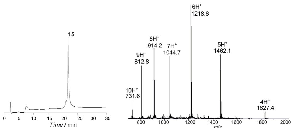
**Figure S28.** Characterization of **15**, the ligation product of **11** with **12**, by analytical RP-HPLC chromatograms ( $\lambda = 214$  nm) and ESI-MS. HPLC conditions: a linear gradient of 20-60% acetonitrile (with 0.08-0.1% TFA) in water (with 0.1% TFA) over 30 min (5% for 2 min, then 20%-
