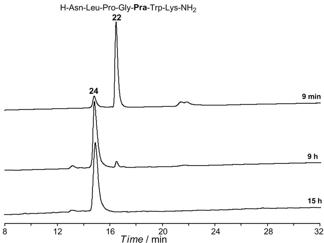
**Figure S18.** The reaction mixture of **22** was monitored by analytical RP-HPLC chromatograms ( $\lambda = 214$  nm). HPLC conditions: a linear gradient of 5-50% acetonitrile (with 0.08-0.1% TFA) in water (with 0.1% TFA) over 30 min (5% for 2 min, then 5%-50% for 30 min) on a Vydac C18 (4.6  $\times$  150 mm) column.
