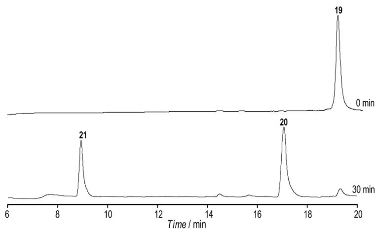
**Figure S26.** Substrate hydrolysis by a commercial HIV-1 protease. The hydrolysis process was monitored by analytic RP-HPLC ( $\lambda = 214$  nm). RP-HPLC conditions: a linear gradient of 5-70% acetonitrile (with 0.08-0.1% TFA) in water (with 0.1% TFA) over 30 min on a Vydac C8 ( $4.6 \times 150$  mm) column. Time points: 0 min and 30 min after the incubation.
