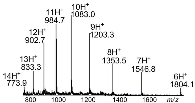
**Figure S31.** The ESI-MS spectrum of protein **18**. The spectrum gave an observed mass of 10820.2 Da (calcd 10820.7 Da, average isotopes).
