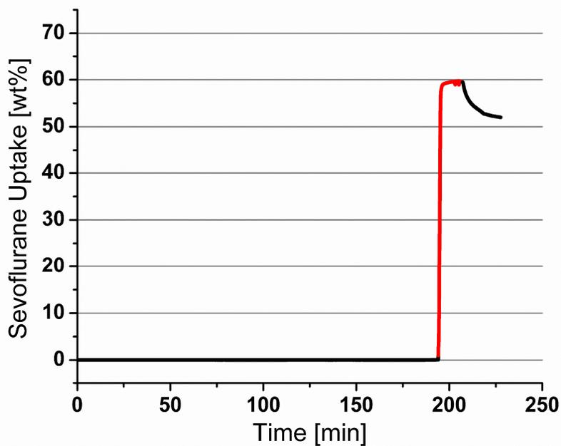
**Figure S4.** TGA trace for adsorption of sevoflurane (**3**) within the pores of **6**. Red trace shows the flow of anesthetic-enriched nitrogen, black trace the flow of pure nitrogen.
