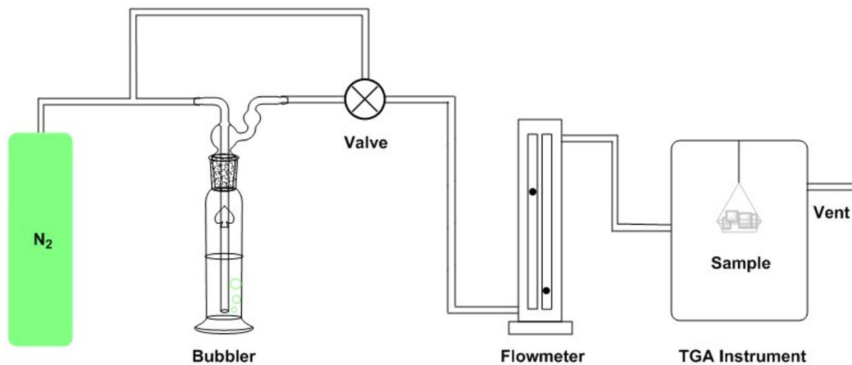
**Figure S1.** A schematic diagram of the apparatus for TGA of anesthetic vapor adsorption.
