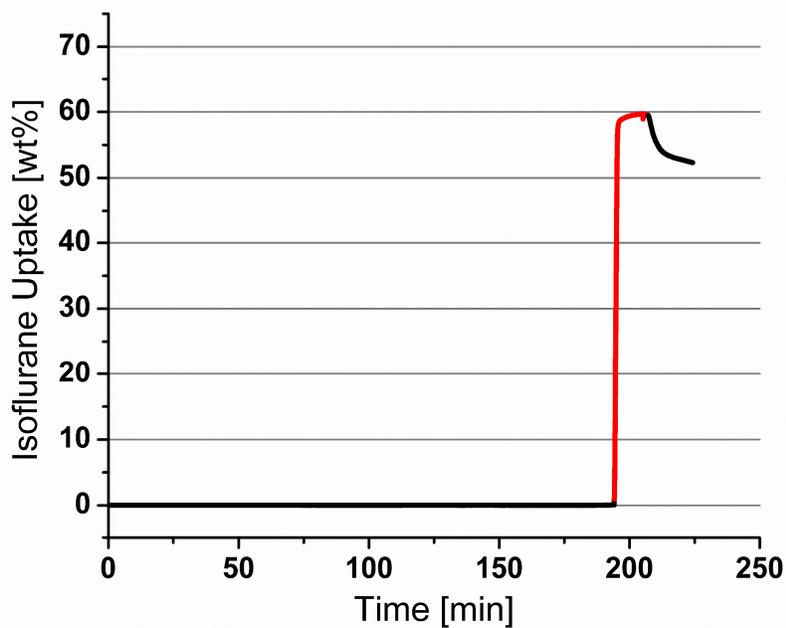
**Figure S3.** TGA trace for adsorption of isoflurane (**2**) within the pores of **6**. Red trace shows the flow of anesthetic-enriched nitrogen, black trace the flow of pure nitrogen.
