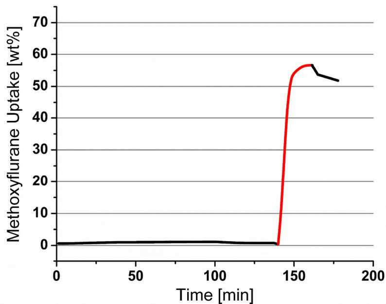
**Figure S5.** TGA trace for adsorption of methoxyflurane (**4**) within the pores of **6**. Red trace shows the flow of anesthetic-enriched nitrogen, black trace the flow of pure nitrogen.
