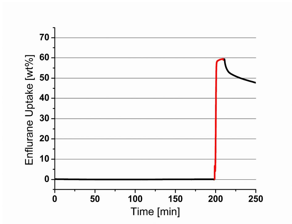
**Figure S2.** TGA trace for adsorption of enflurane (1) within the pores of 6. Red trace shows the flow of anesthetic-enriched nitrogen, black trace the flow of pure nitrogen.
