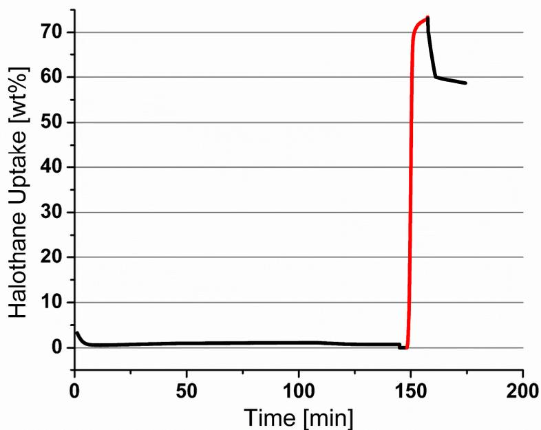
**Figure S6.** TGA trace for adsorption of halothane (**5**) within the pores of **6**. Red trace shows the flow of anesthetic-enriched nitrogen, black trace the flow of pure nitrogen.
