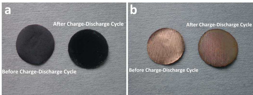
**Fig. S2** Photographs of the test electrodes before and after charge-discharge cycles: (a) One side with active material  $\text{CH}_3\text{NH}_3\text{PbBr}_3$ . (b) The other side of the Cu foil with diameter of 14 mm.
