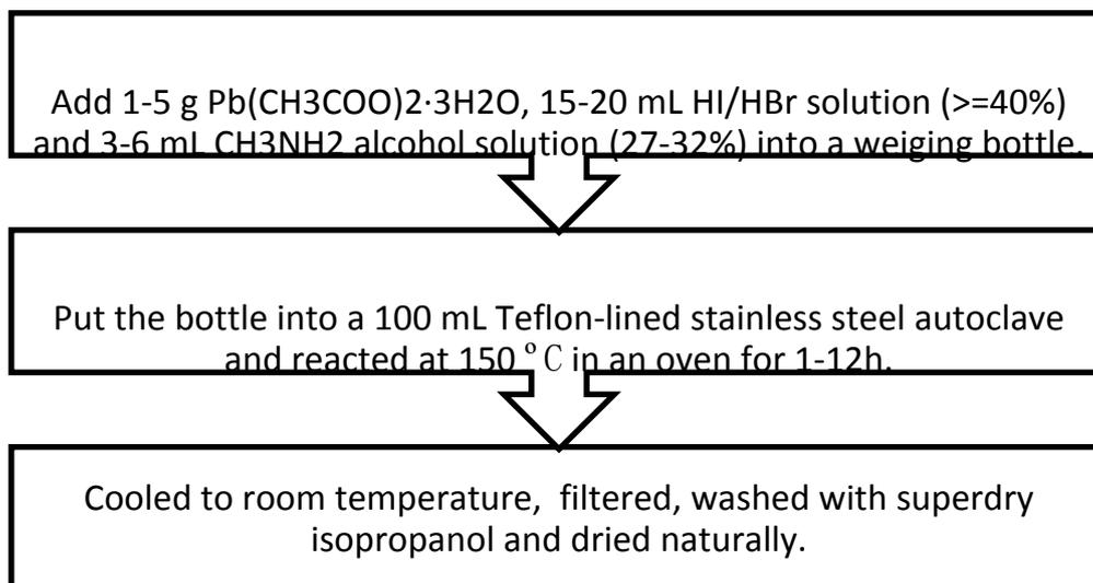
**Scheme S1.** Synthesis process of the perovskite  $\text{CH}_3\text{NH}_3\text{PbX}_3$ .
