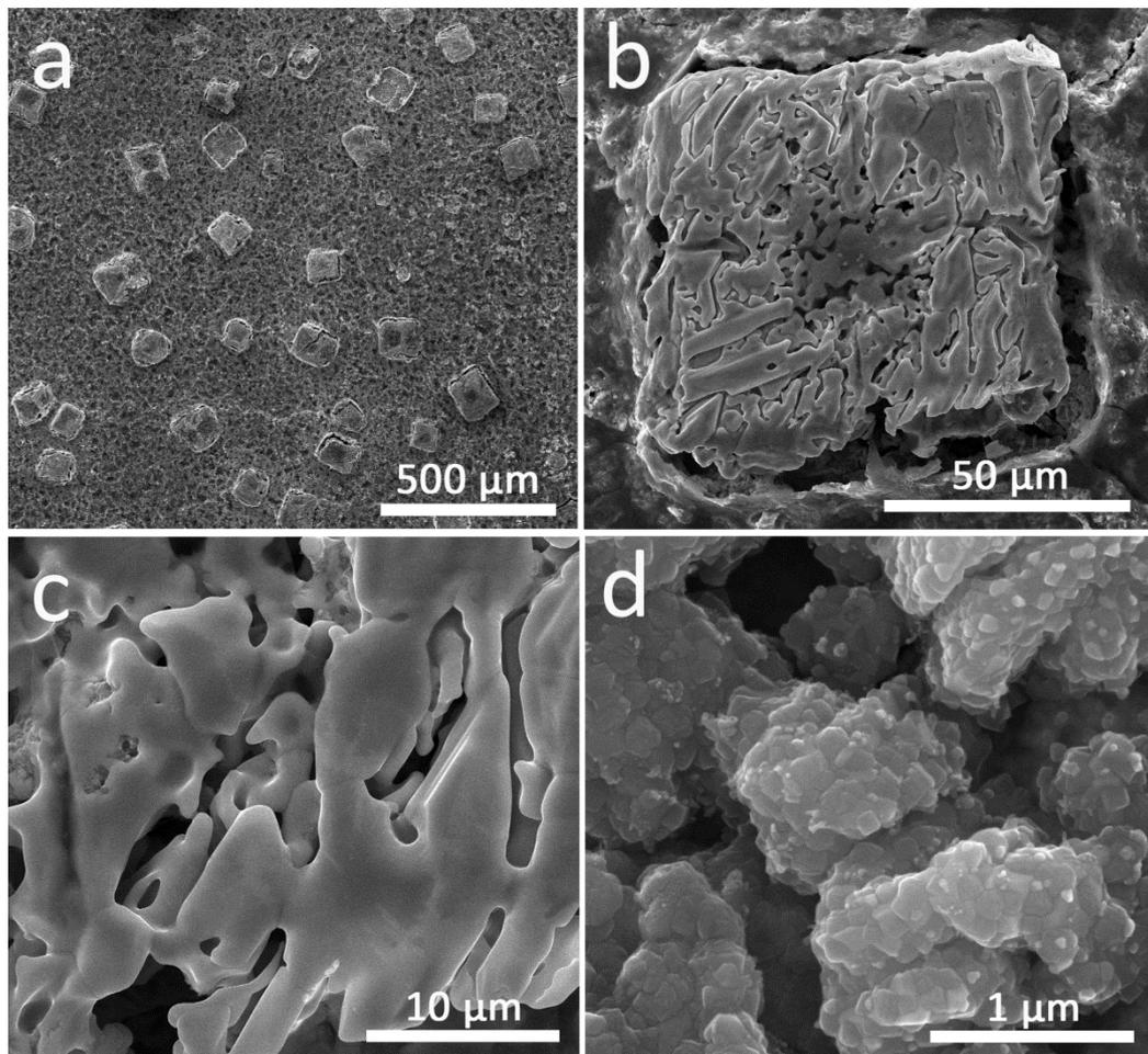
**Fig. S1** SEM images of the as-prepared  $\text{CH}_3\text{NH}_3\text{PbBr}_3$  test electrode with different magnifications (scale bar: 500  $\mu\text{m}$  for a, 50  $\mu\text{m}$  for b, 10  $\mu\text{m}$  for c, 1  $\mu\text{m}$  for d).
