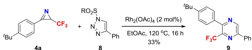
An oven-dried tube was charged with 2*H*-azirines **4a** (0.2 mmol), N-sulfonyl-4-phenyl-1,2,3-triazole **8**, and  $\text{Rh}_2(\text{OAc})_4$  (0.004 mmol). Then,  $\text{EtOAc}$  (1.0 mL) was added into the tube. The reaction mixture was stirring at  $120$   $^\circ\text{C}$  for 16 h (monitored by thin-layer chromatography using silica gel precoated glass plates), concentrated in vacuum and purified by flash column chromatography (silica gel) to afford the product **9**.
