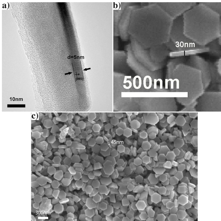
**Figure S3.** TEM and SEM images of Cu<sub>2</sub>S nanoplates with different thicknesses: a) 5 nm; b) 30 nm; c) 45 nm.
