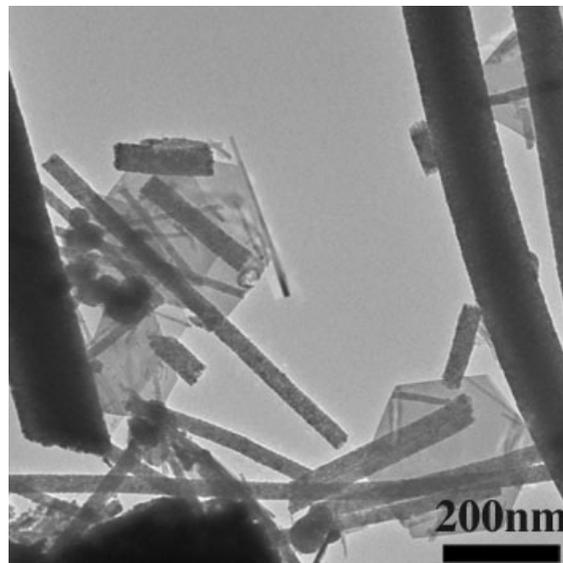
**Figure S5.** TEM image of Cu<sub>2</sub>S NS/TiO<sub>2</sub>
