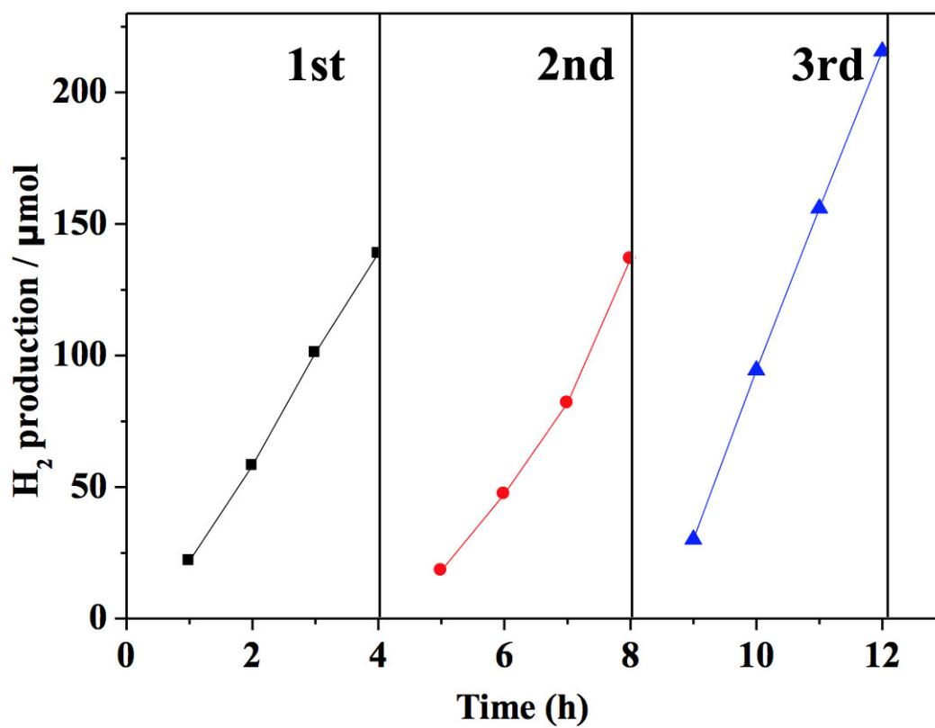
Figure S6. Time course of photocatalytic H<sub>2</sub> production over Cu<sub>2</sub>S NS/TiO<sub>2</sub>.
