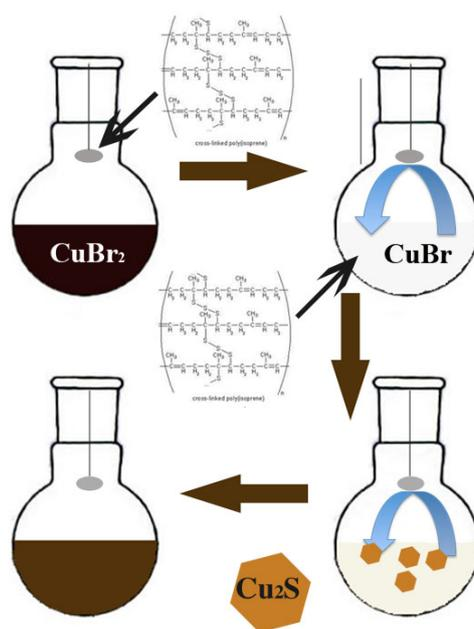
**Scheme S1.** Schematic diagram of the formation process of Cu<sub>2</sub>S NS.
