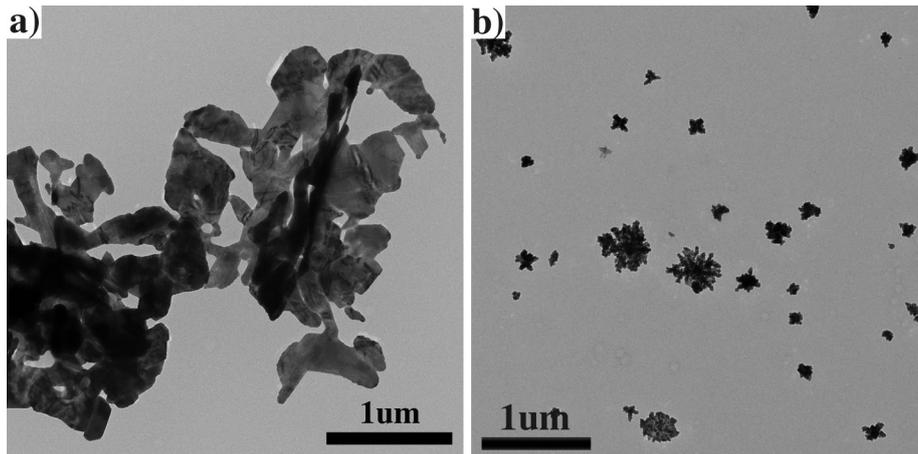
**Figure S2.** TEM images of Cu<sub>2</sub>S synthesized with different precursors: a) sulfur powder; b) thiourea.
