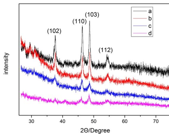
**Figure S1.** XRD patterns of Cu<sub>2</sub>S nanoplates with different thicknesses: a) 45 nm; b) 30 nm; c) 5 nm; and d) 1.2 nm.
