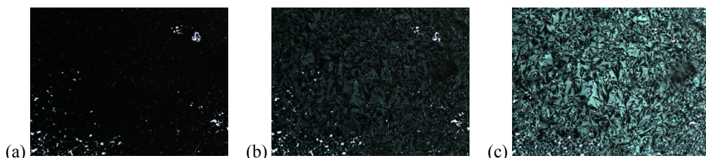
Fig. S1. Polarized photomicrographs of (a) a homeotropic domain formed by QL32-6 in the SmA* phase at 63 °C, and developing Schlieren texture in the same domain upon transition to the SmC* phase at (b) 61 °C and (c) 51 °C.
