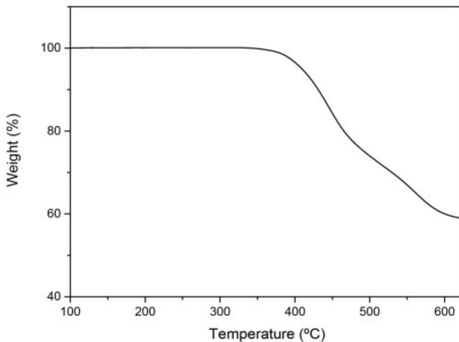
**Figure S1.** Thermogravimetric Analysis of **TAE-1** at scan rate of 10 °C/min
