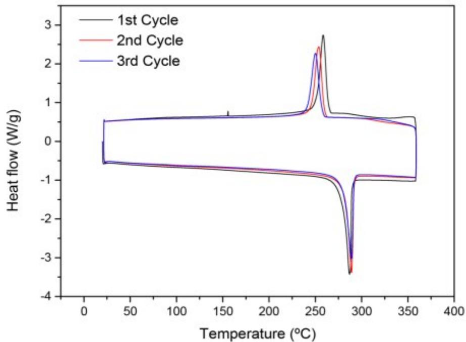
**Figure S2.** Differential Scanning Calorimetry of **TAE-1** with scan rate of 20 °C/min
