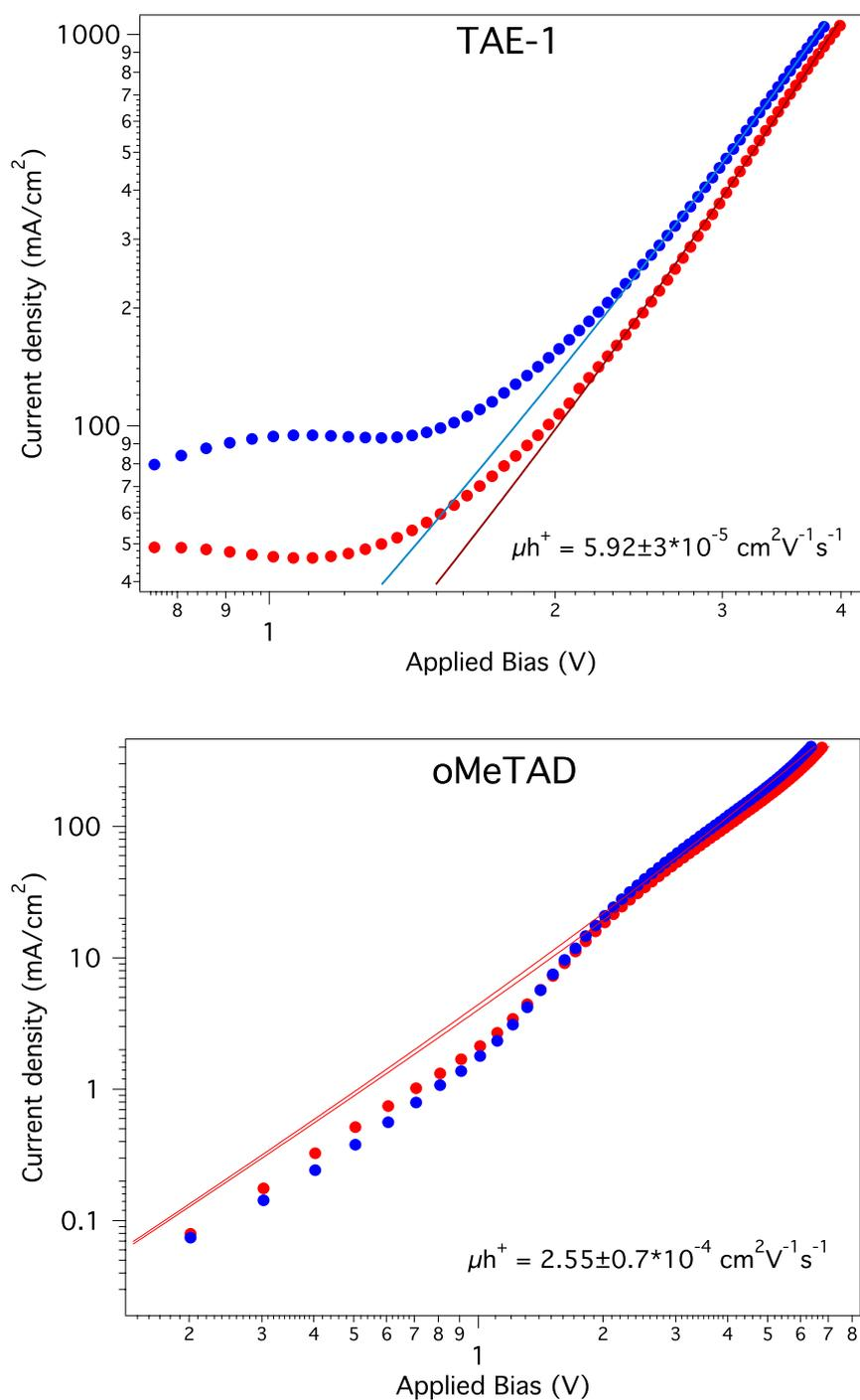
**Figure S3:** Hole only **TAE-1** (up), Spiro-OMeTAD (down) devices J-V at space charge limited conditions. The red symbols correspond to the measurement under illumination and the blue symbols correspond to the measurement under dark.
