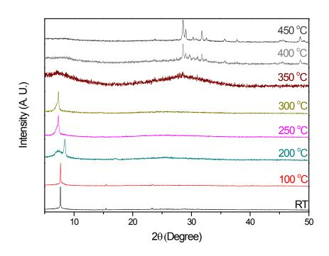
S4. Energy dispersive analysis by X-ray (EDX) data and powder X-ray diffraction pattern for the product of competing crystallization reaction between Cd<sup>2+</sup> and Pb<sup>2+</sup> with Kemp's triacid
