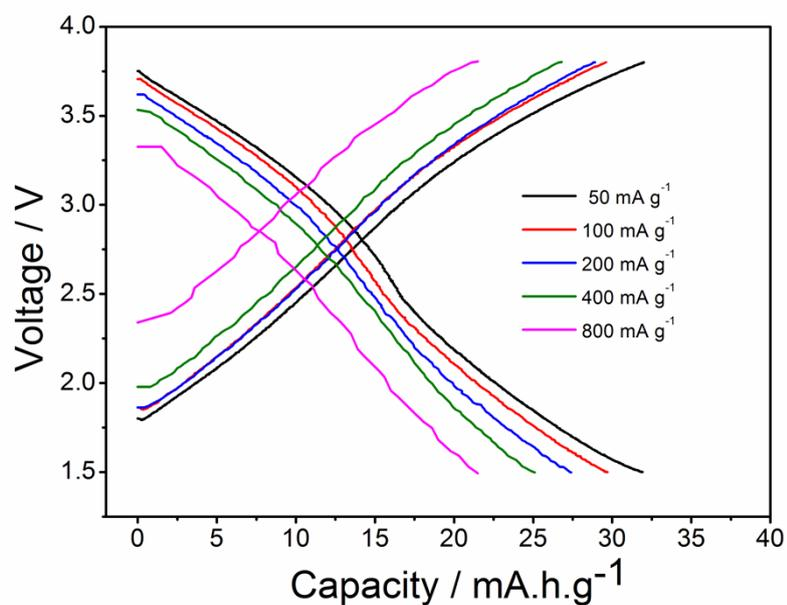
**Figure S6.** The charge-discharge profiles of KB electrode in 1.0 mol L<sup>-1</sup> NaPF<sub>6</sub> +EC-DEC (v/v=1/1) electrolyte at various current densities in a voltage range of 1.5 to 3.8 V.
