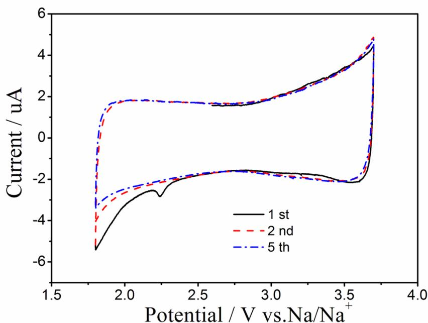
**Figure S5.** CV curves of the carbon additive (KB) measured in  $1.0 \text{ mol L}^{-1} \text{ NaPF}_6 + \text{EC-DEC}(\text{V}:\text{V}=1:1)$  electrolyte in a voltage range of 1.8 to 3.7 V. Scan rate:  $0.2 \text{ mV s}^{-1}$
