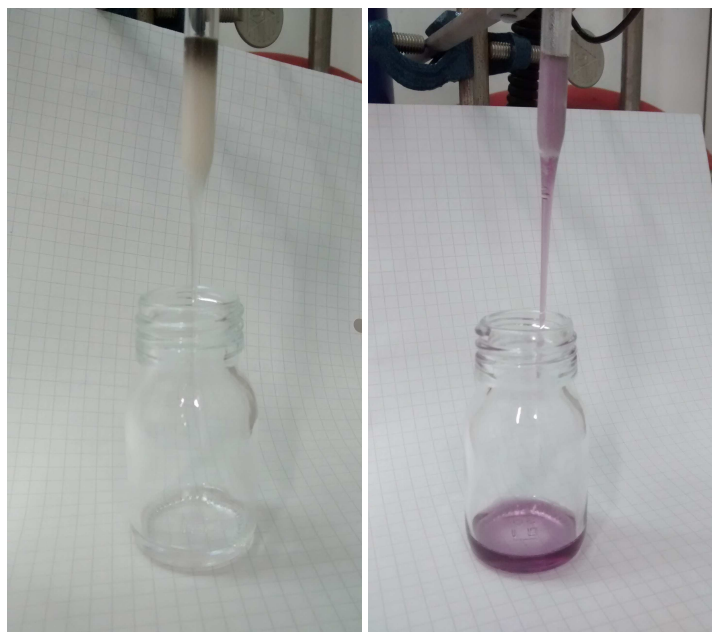
Fig. S3 Adsorption experiments of a solution of Pt nanoparticles (left) and \text{Pt}(\text{dba})_2 (right) on a Celite® plug.
