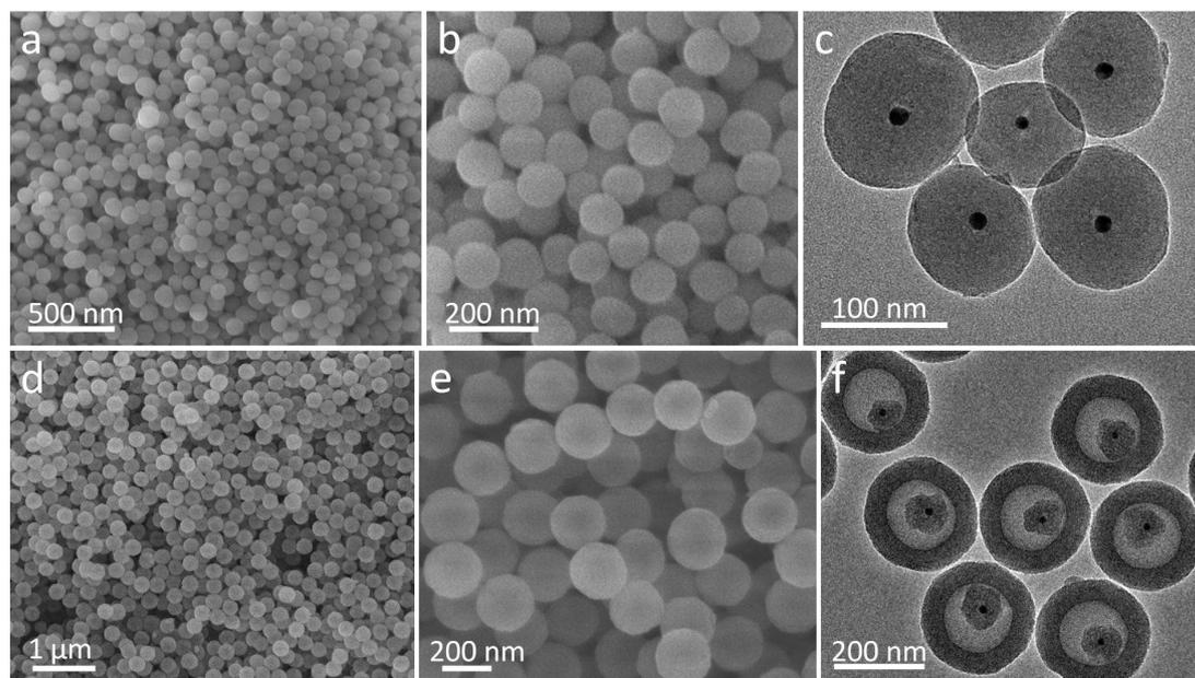
**Figure S1.** SEM and TEM images of core-shell structured Au@SiO<sub>2</sub> (a, b, c) and yolk-shell structured Au@SiO<sub>2</sub>@Ph-PMO (d, e, f).
