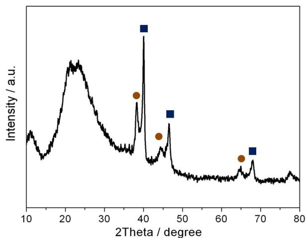
**Figure S6.** Wide-angle XRD pattern of amphiphilic nanoreactor Au@Pd@Ph-PMO. The diffraction peaks at  $2\theta$  values of approximately 40.0, 46.5 and 67.9 degrees (directed by ■) in the wide-angle XRD pattern are attributed to the crystalline Pd nanoparticles.
