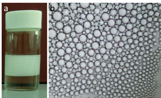
**Figure S5.** (a) Digital photograph of water in oil emulsion in toluene-water system obtained using surfactant CTAB as emulsifier. (b) Microphotograph of the water in oil emulsion in (a).
