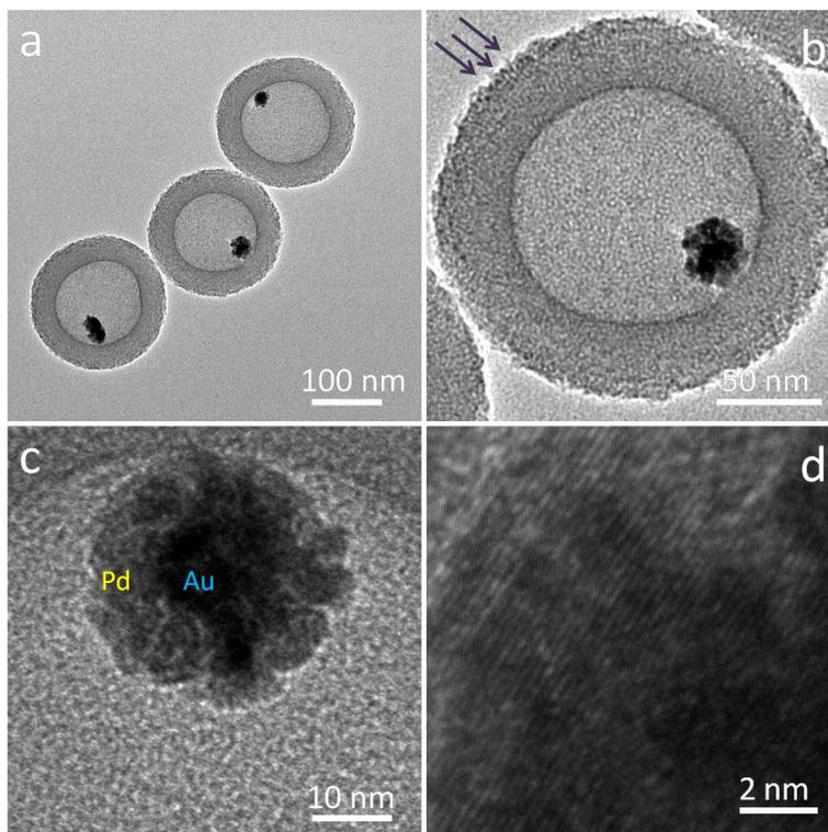
**Figure S10.** Low-magnification and high-magnification TEM images of hydrophilic nanoreactor Au@Pd@SiO<sub>2</sub>. These images indicate that this hydrophilic nanoreactor Au@Pd@SiO<sub>2</sub> has the identical structural property including the unique yolk-shell nanostructure, the oriented mesochannels in external shell and the catalytically active Au@Pd bimetal structure with the amphiphilic nanoreactor Au@Pd@Ph-PMO.
