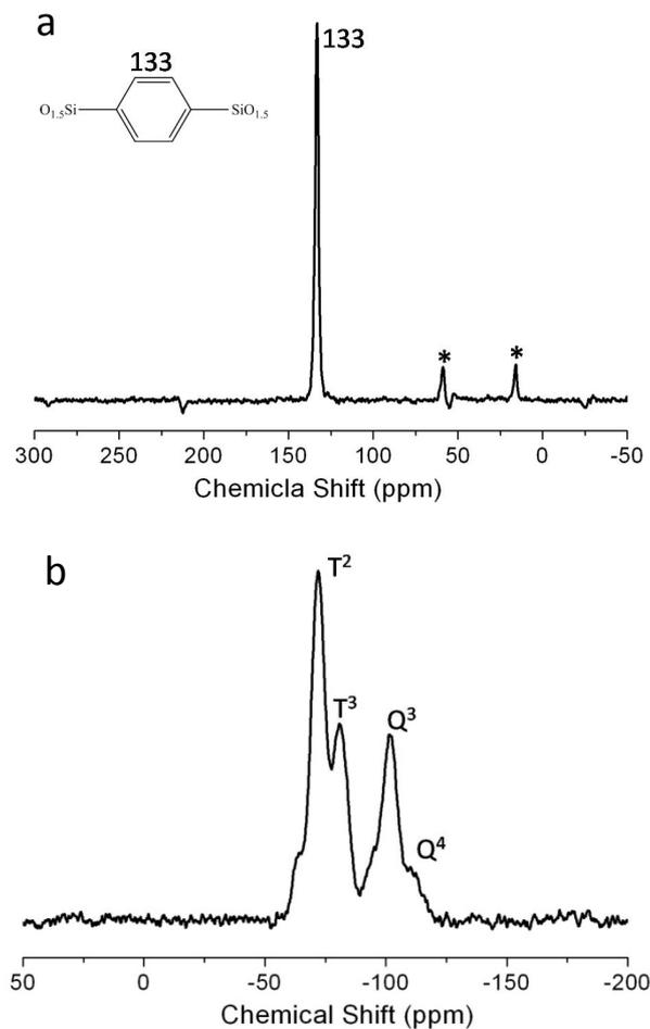
**Figure S4.** Solid-state  $^{13}\text{C}$  NMR (a) and  $^{29}\text{Si}$  NMR (b) spectroscopy of yolk-shell structured Au@Ph-PMO.
