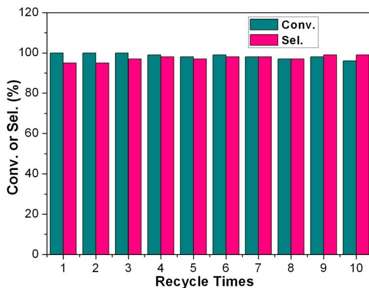
**Figure S8.** Recycling runs for the aerobic oxidation of 4-methoxybenzyl alcohol by Au@Pd@Ph-PMO catalyst. Reaction condition: 4-methoxybenzyl alcohol (0.5 mmol), K<sub>2</sub>CO<sub>3</sub> (0.5 mmol, 1 equi), 4 mL of H<sub>2</sub>O, catalyst (Pd 1.5 mol%), open air, 5 h.
