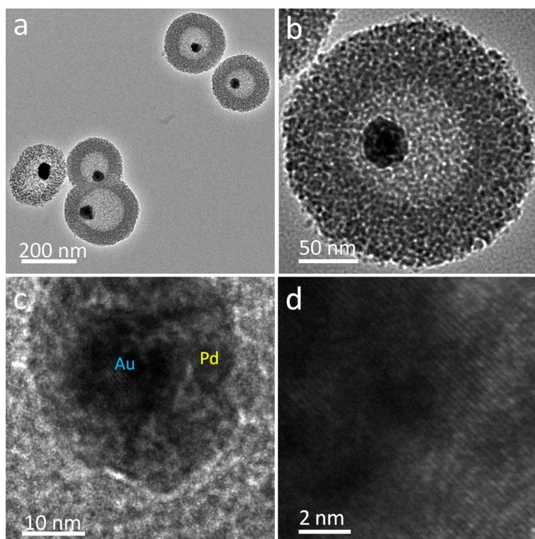
**Figure S9.** Low-magnification and high-magnification TEM images of amphiphilic nanoreactor Au@Pd@Ph-PMO recovered after successive recycling ten times for oxidation of 4-methoxybenzyl alcohol.
