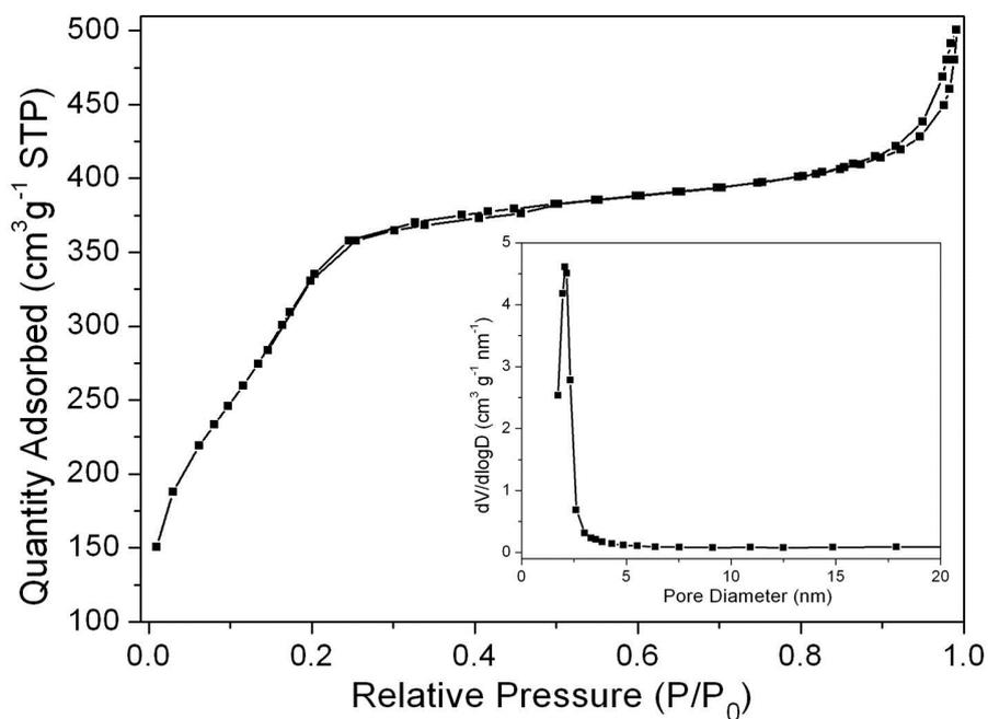
**Figure S3.** Nitrogen sorption isotherm and BJH pore size distribution curve (the inset) of yolk-shell structured Au@Ph-PMO.
