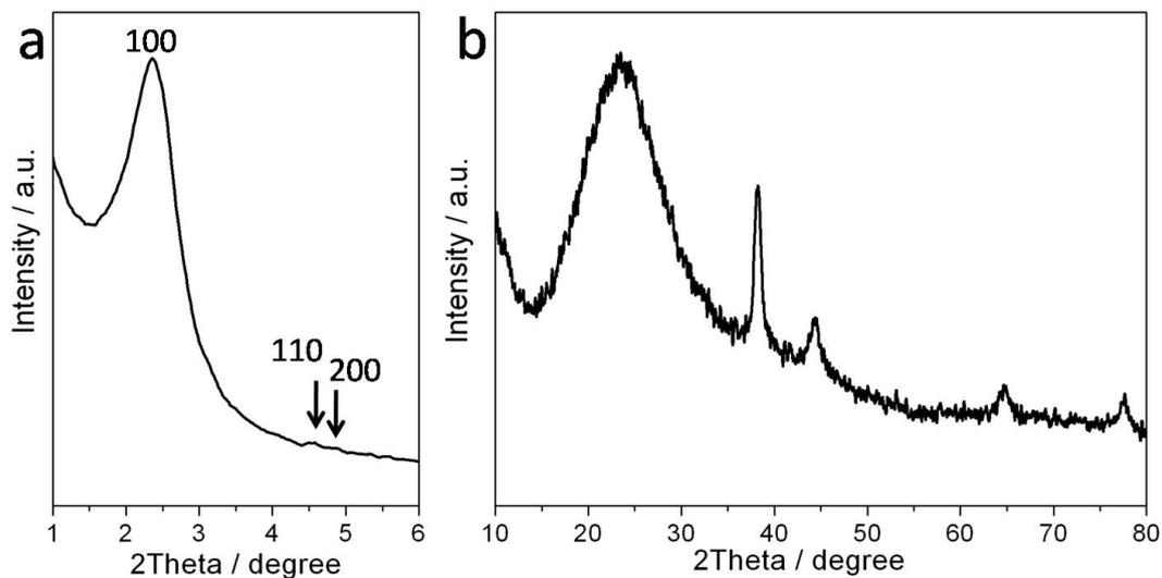
**Figure S2.** Small- and wide-angle XRD patterns of yolk-shell structured Au@Ph-PMO. The diffraction peaks at  $2\theta$  values of approximately 38.2, 44.3, 64.7 and 77.6 degrees in the wide-angle XRD pattern (b) are attributed to the Au nanoparticles.
