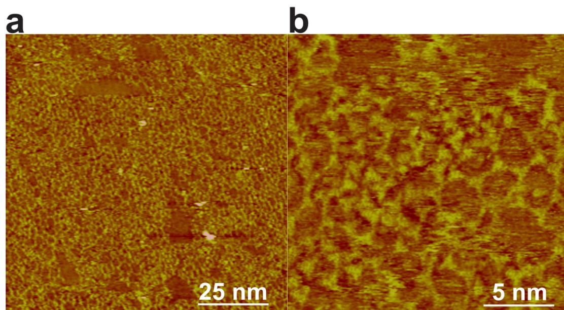
Fig. S1. STM images of  $s\text{COF}_{\text{C+D}}$  fabricated at 60 °C. (a) Large-scale STM image ( $100 \times 100 \text{ nm}^2$ ) of  $s\text{COF}_{\text{C+D}}$ . (b) High resolution STM image ( $20 \times 20 \text{ nm}^2$ ) of  $s\text{COF}_{\text{C+D}}$ . Imaging conditions: (a)  $V_{\text{bias}} = 700 \text{ mV}$ ,  $I_t = 500 \text{ pA}$ ; (b)  $V_{\text{bias}} = 700 \text{ mV}$ ,  $I_t = 650 \text{ pA}$ .
