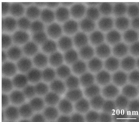
**Fig. S2** SEM image of patterned Ti surface after removed the first-anodized TiO<sub>2</sub> NTs.
