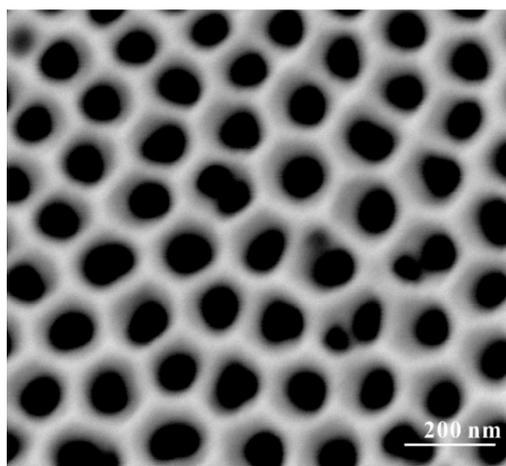
**Fig. S4** SEM image of TiO<sub>2</sub> NTs.
