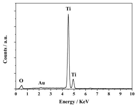
**Fig. S5** EDS of Au/SD-TiO<sub>2</sub> NTs.
