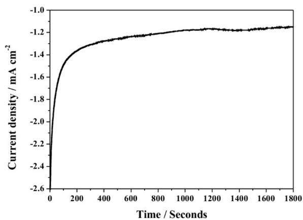
**Fig. S3** I-t curve of electrochemical reduction of TiO<sub>2</sub> NTs at -1.5 V vs Ag/AgCl.
