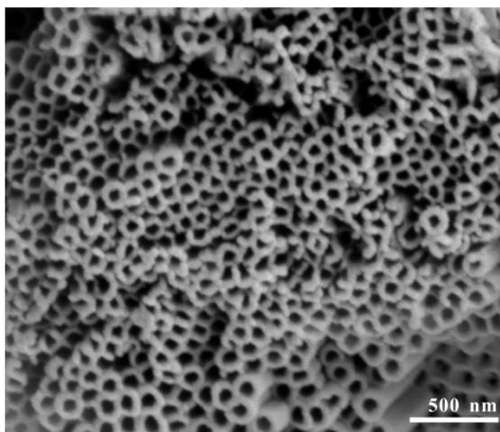
**Fig. S1** SEM image of first-step anodized TiO<sub>2</sub> NTs.
