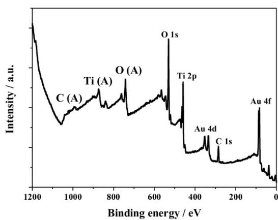
**Fig. S6** XPS survey of Au/SD-TiO<sub>2</sub> NTs.
