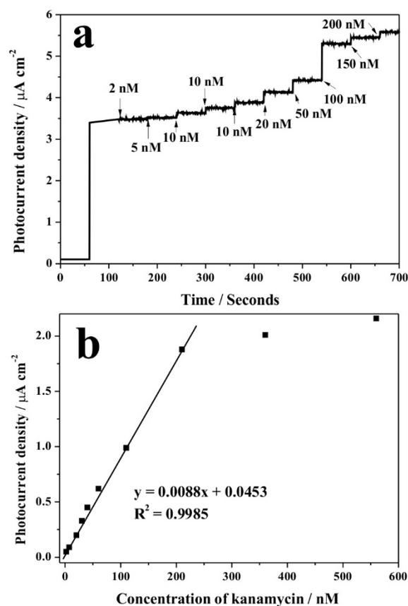
**Fig. S8** (a) Photocurrent density vs time for successive addition of kanamycin at 0.5 V vs Ag/AgCl under illumination of visible light with wavelength  $\geq 420$  nm on aptamer-Au/TiO<sub>2</sub> NTs; (b) photocurrent density-kanamycin concentration calibration curve on aptamer-Au/TiO<sub>2</sub> NTs.
