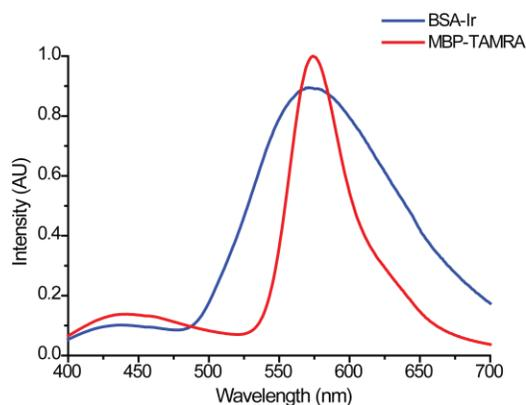
**Figure S4.** Steady-state emission curves of BSA-Ir (blue line) and MBP-TAMRA (red line) on blot membrane. Both compounds were excited at 370 nm. The broad, weak emission near 450 nm was observed even for blank membrane.
