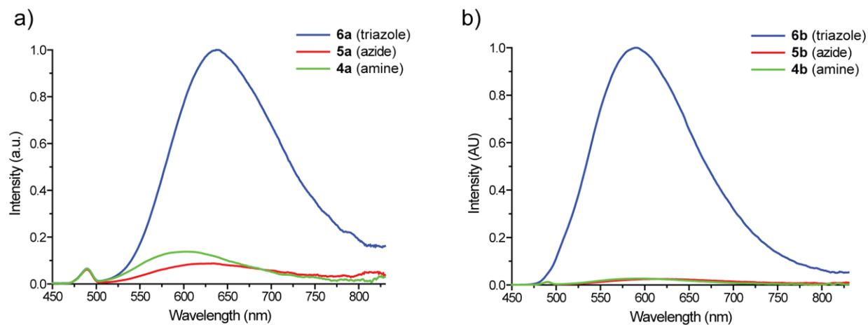
**Figure S2.** Emission spectra of a) complexes **4a**, **5a**, and **6a** in PBS buffer/MeOH (4:1) b) carboxylate-containing complexes **4b**, **5b**, and **6c** in PBS buffer/MeOH (95:5). All complexes were excited at 420 nm.
