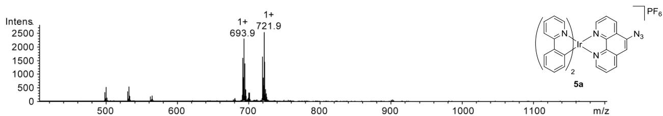
**Figure S10.** Parent azide complex **5a** (positive mode).  $m/z$  721.9 and 693.9 correspond to  $[M]^+$  and  $[M-N_2]^+$ , respectively.
