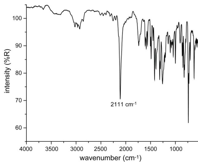
**Figure S8.** IR spectrum of 5-azidophenanthroline **3**. An azide stretch was observed at 2111 cm<sup>-1</sup>.
