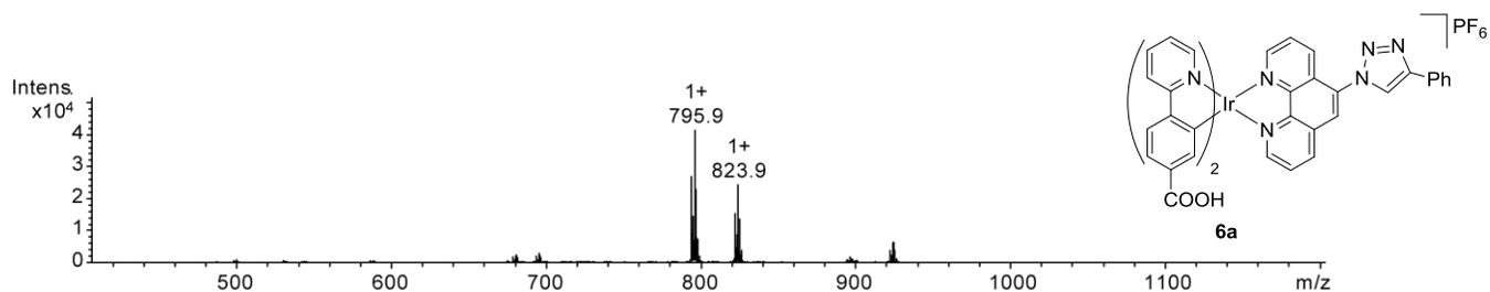
**Figure S14.** Parent triazole complex **6a** (positive mode).  $m/z$  823.9 and 795.9 correspond to  $[M]^+$  and  $[M-N_2]^+$ , respectively.
