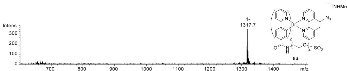
**Figure S13** Bisulfate azide complex **5d** (negative mode).  $m/z$  1317.7 corresponds to  $[M]^-$ .
