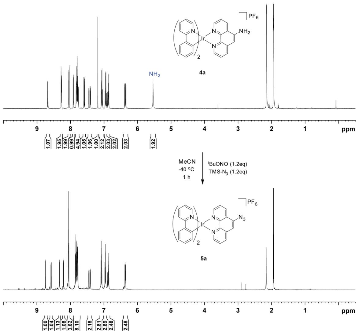
**Figure S7.**  $^1\text{H}$  NMR spectra of parent amine complex **4a** and azide complex **5a** in  $\text{CD}_3\text{CN}$ . Upon conversion of amine to azide group, a broad peak at 5.5 ppm disappeared.
