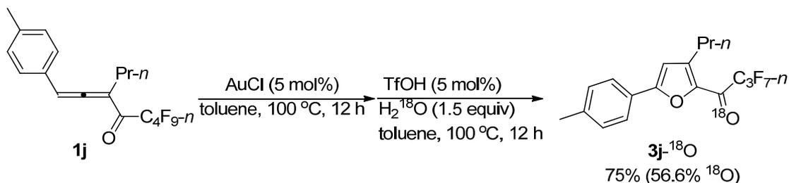
To a dried Schlenk tube were added anhydrous AuCl (97%, 0.0025 g, 0.010 mmol), 1-(4'-methylphenyl)hexa-1,2-dien-3-yl perfluorobutyl ketone **1j** (0.0831 g, 0.20 mmol), and anhydrous toluene (2 mL) at room temperature under N<sub>2</sub> atmosphere. The resulting mixture was then placed in a pre-heated oil bath of 100 °C and stirred.
