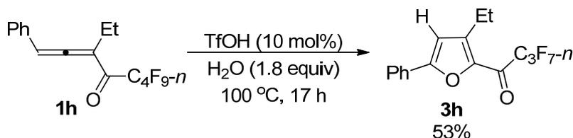
The reaction of 1-phenylpenta-1,2-dien-3-yl perfluorobutyl ketone **1h** (0.1946 g, 0.50 mmol) with TfOH (99%, 4.5  $\mu$ L,  $d = 1.695$  g/mL, 0.0076 g, 0.05 mmol) and H<sub>2</sub>O (16.2  $\mu$ L,  $d = 1.0$  g/mL, 0.0162 g, 0.90 mmol) at 100 °C for 17 h to afford **3h** (0.0966 g, 53%) (petroleum ether/ethyl acetate = 500/1) as a solid: m.p. 40.2-41.2 °C
