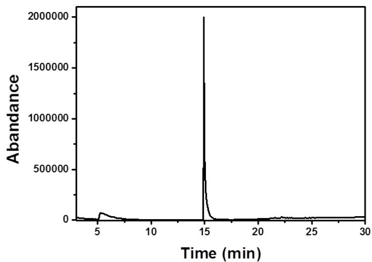
**Fig S3.** Gas chromatography analysis of pFS-DT after treatment with H<sub>2</sub>O<sub>2</sub>. Main decomposition product at Rt 15 min was assigned as diethyl 2,5-dihydroxyterephthalate (DT); MS (*m/z*, %): 255 (*M*+1, 5), 254 (*M*<sup>+</sup>, 31), 209 (27), 208 (100), 181 (5), 180 (22), 163 (13), 162 (72), 135 (7), 134 (15), 107 (9), 79 (5), 78 (5), 53 (9).
