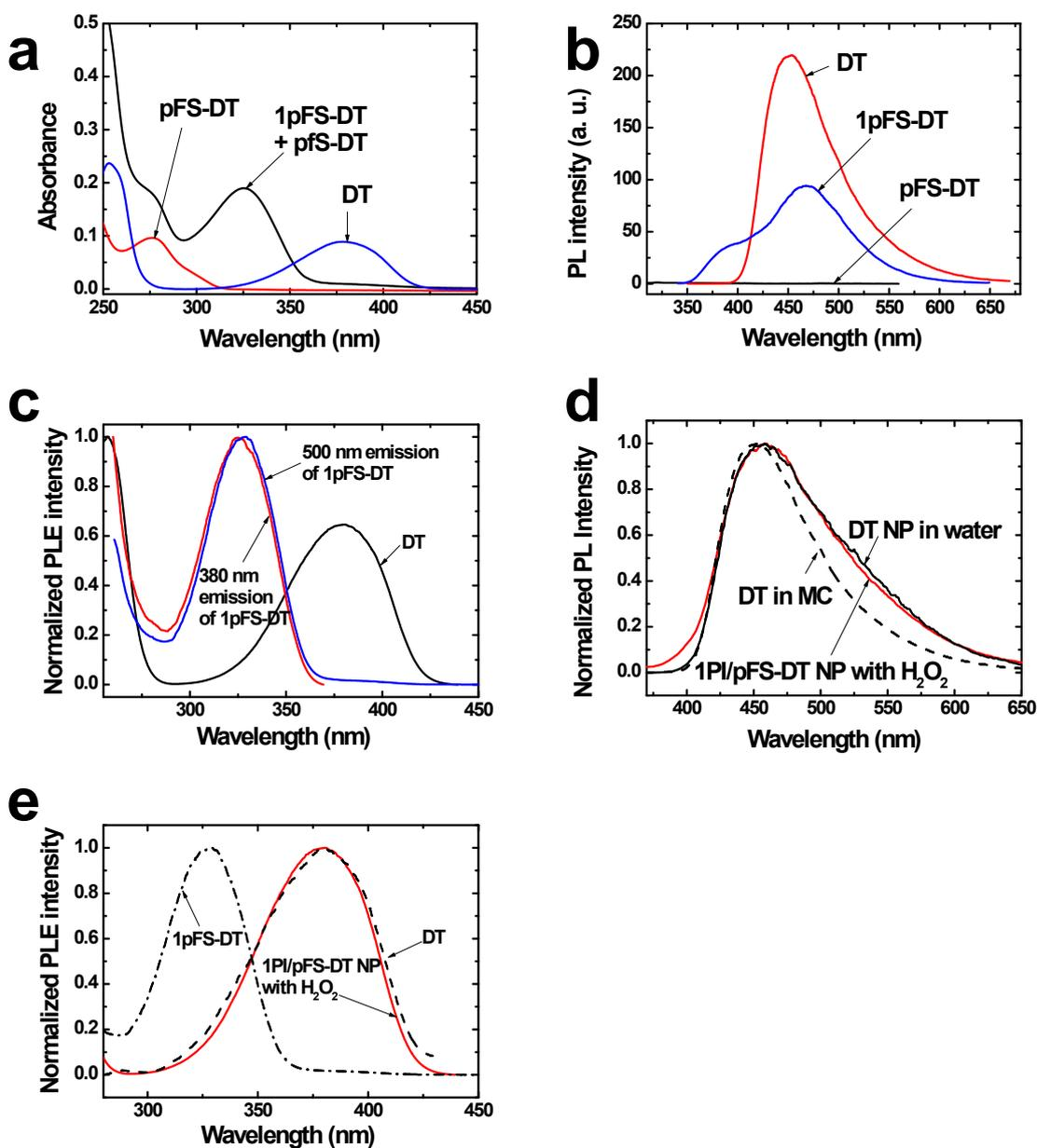
**Fig S2.** (a) Absorption spectra of pFS-DT, 1pFS-DT (mixture) and DT. (b) Fluorescence spectra of pFS-DT, 1pFS-DT (mixture) and DT. (c) Excitation spectra for the fluorescence of DT and 1pFS-DT (mixture). (d) Fluorescence spectra of DT (in dichloromethane, MC), DT NPs (in water) and 1PI/pFS-DT NPs (in water) reacted with  $H_2O_2$ . (e) Excitation spectra for the fluorescence of DT, 1pFS-DT (mixture) and 1PI/pFS-DT NPs reacted with  $H_2O_2$ .
