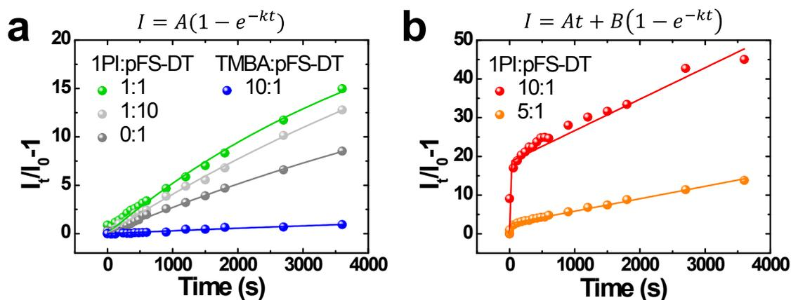
**Fig S4.** Kinetic profiles for  $\text{H}_2\text{O}_2$  sensing of NPs with different types and amounts of the catalyst.  $I_t$  is fluorescent intensity at a given time  $t$ , and  $I_0$  is initial fluorescent intensity before  $\text{H}_2\text{O}_2$  addition. Solid lines are fitted with equations for pseudo-first-order kinetics in (a) and pre-steady-state burst kinetics in (b).
