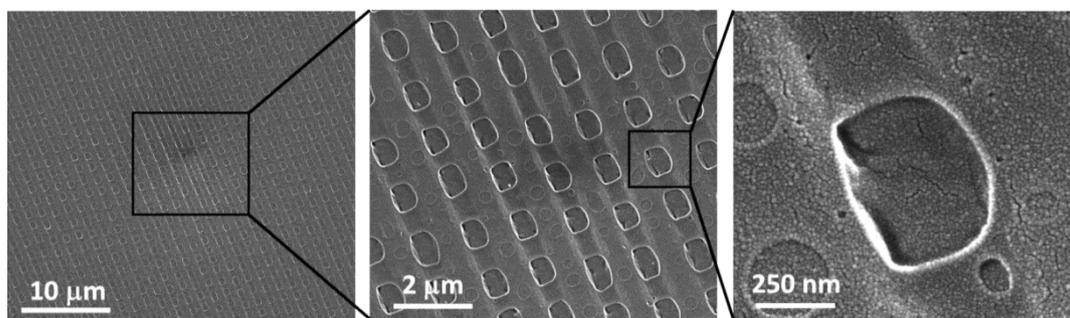
**Supporting Information Figure S7.** SEM images of the deposited sulfur on CD-ROM surface at a relative high temperature of 172 °C with varying deposition time: (A) 10 s, (B) 30 s and (C) 60 s.
