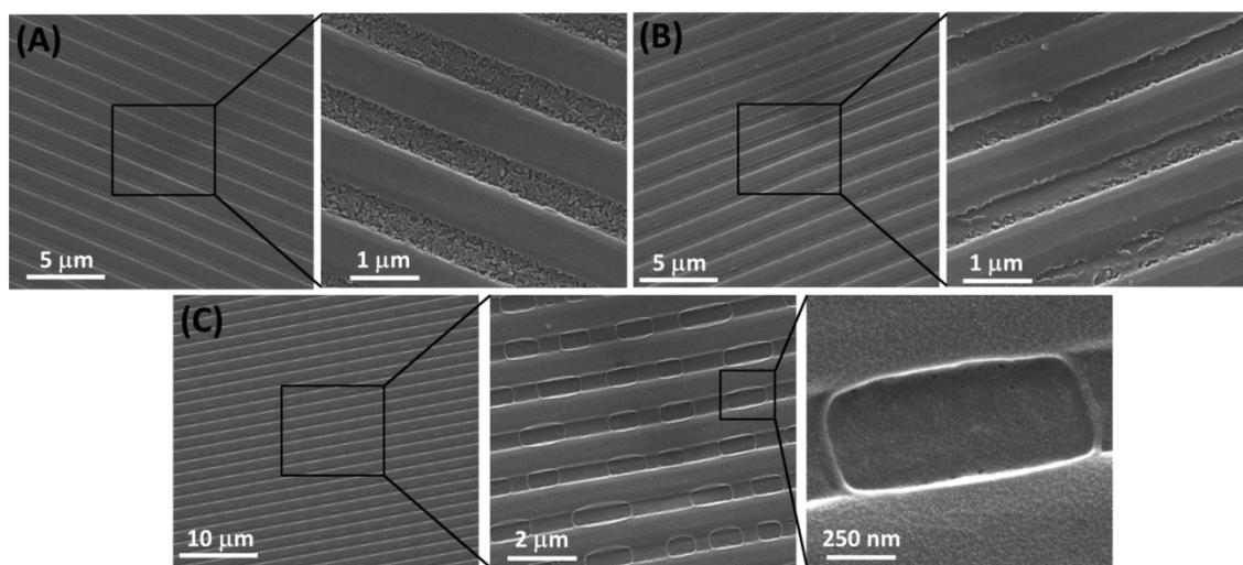
**Supporting Information Figure S6.** SEM images of the deposited sulfur pattern formed on CD-ROM surface with an optimal condition: 150 °C for 60 s.
