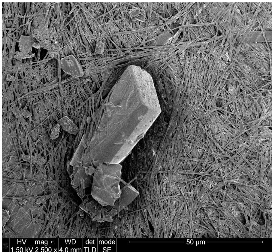
Figure S2 SEM image of a xerogel of 1a obtained from nitromethane showing a mixture of fibres and solid crystalline particles.
