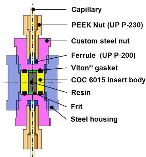
**Fig. S4:** Schematic of miniaturized QMA (10 mg) setup located external to the chip.
