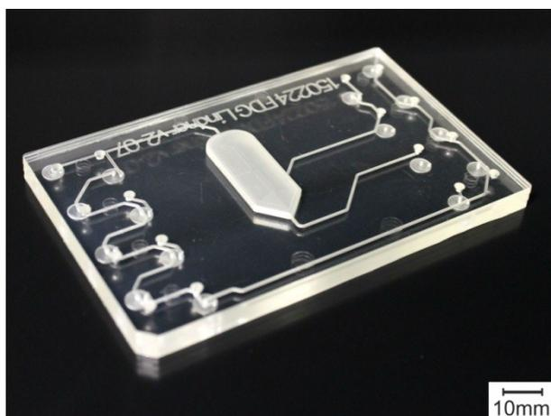
**Fig. S3:** Microfluidic chip utilized for fluid handling and radiolabeling of [<sup>18</sup>F]FTAG
