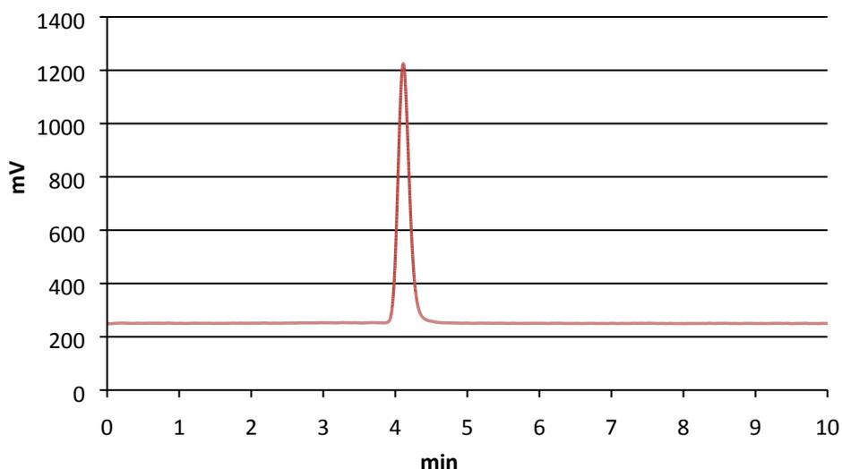
**Fig. S2:** Representative HPLC trace of the purified [<sup>18</sup>F]FDG.
