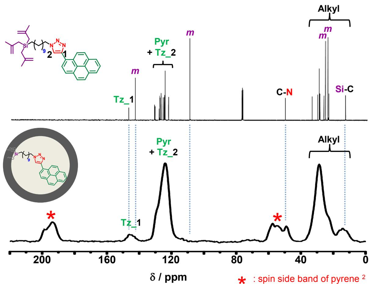
**Figure S2.**  $^{13}\text{C}$  NMR spectrum of **1a** (upper) and  $^{13}\text{C}$  CP-MAS solid state NMR spectrum of **Pyr@Si(15%)** (lower). Peaks marked *m*, which correspond to the methallyl group in **1a** are not present in the spectrum of **Pyr@Si(15%)**.
