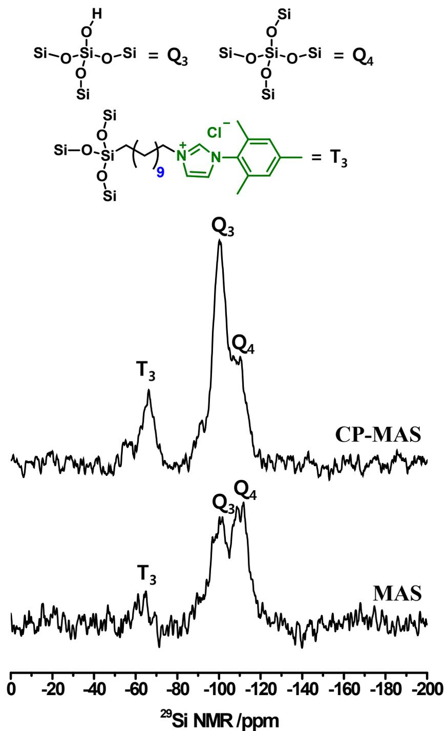
**Figure S5.**  $^{29}\text{Si}$  CP-MAS (top) and MAS (bottom) solid state NMR spectrum of **Imid@Si**. Peaks marked  $\text{Q}_3$  and  $\text{Q}_4$  correspond to the silanol group and the silicate group, respectively. Peaks marked  $\text{T}_3$  correspond to the functional group-impregnated silane group in **Imid@Si**.
