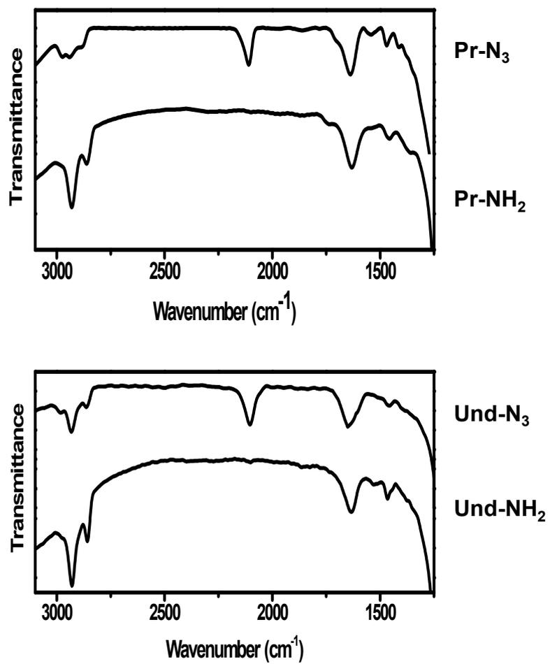
**Figure S3.** FT-IR data for **Pr-NH<sub>2</sub>@Si** and **Und-NH<sub>2</sub>@Si** synthesized from **Pr-N<sub>3</sub>@Si** and **Und-N<sub>3</sub>@Si**.
