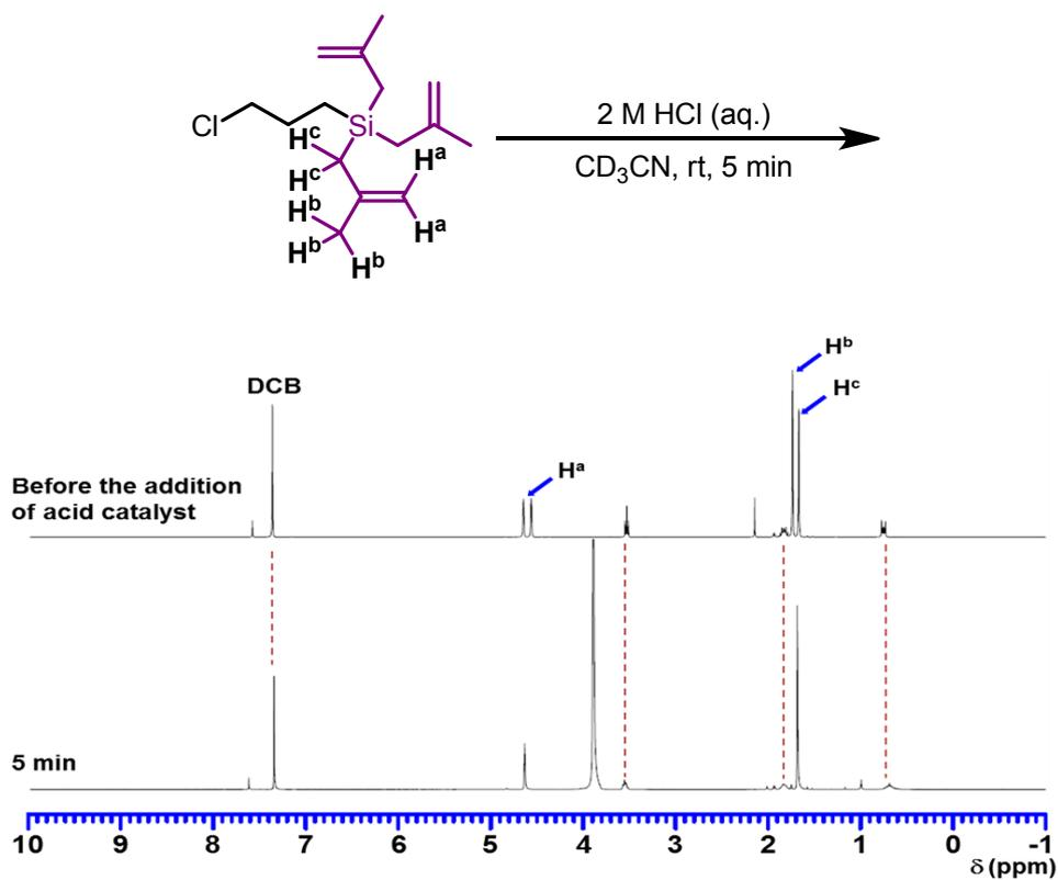
**Figure S1.** NMR monitoring of dissociation of methallyl groups under acidic conditions. Dichlorobenzene (DCB) was used as an internal standard.
