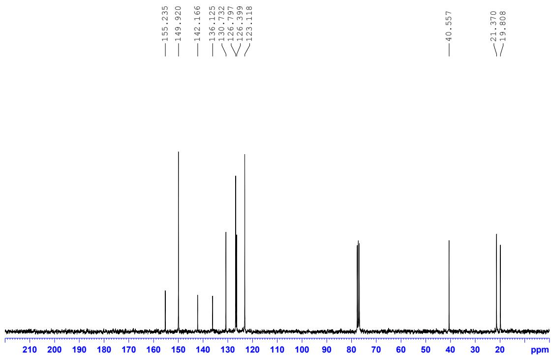
**Figure 70S.**  $^{13}\text{C}\{^1\text{H}\}$  NMR spectrum of **6ab**.
