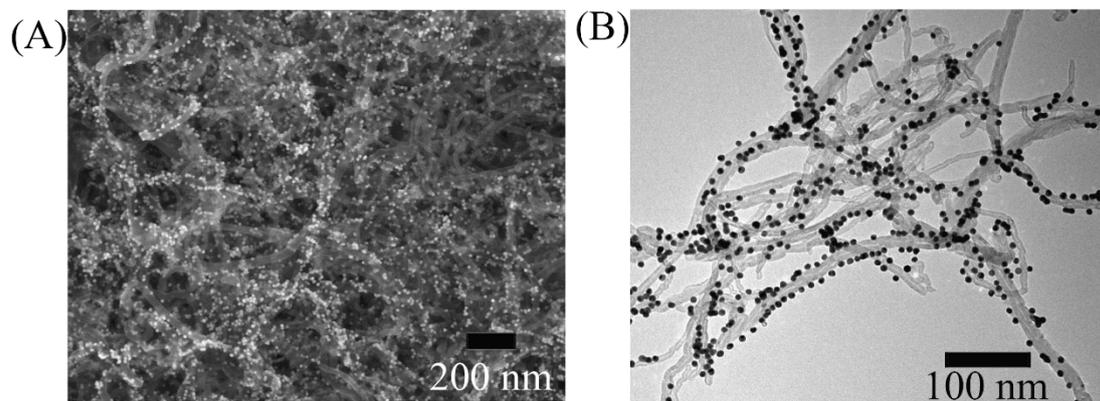
**Fig. S2** SEM (A) and TEM (B) of CNTs/Au NPs
