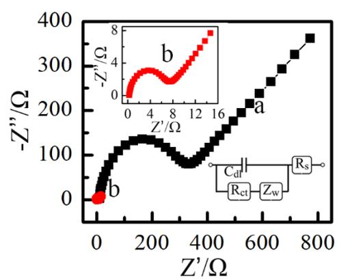
**Fig. S1** EIS of the bare carbon cloth electrode (a) and G/CNTs/Au NPs hybrid modified carbon cloth electrode (b) Insets are the enlarged view of curve b (left) and the Randles equivalent circuit used to fit the EIS data (right).
