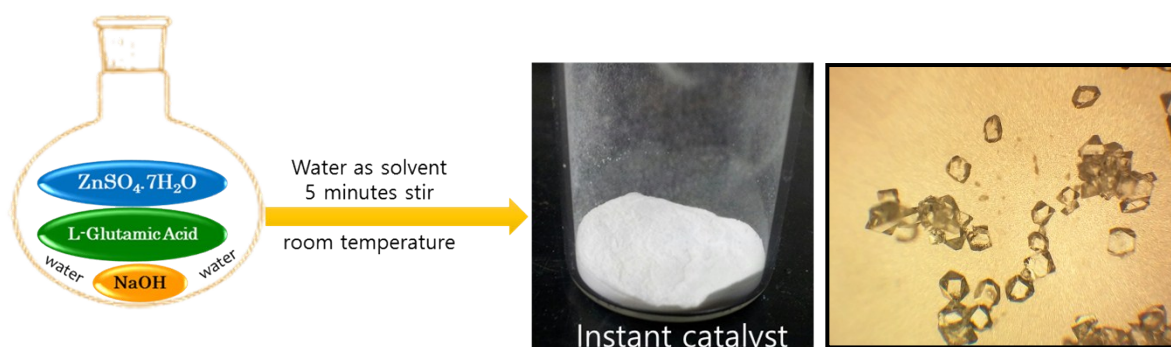
Fig. S1: Scheme for the synthesis of ZnGlu at room temperature, and the images of room temperature synthesized MOF compared with the single crystals (right).
