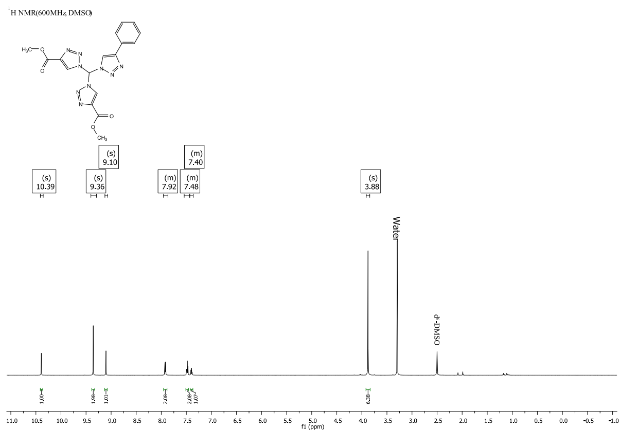
dimethyl 1,1'-((4-phenyl-1H-1,2,3-triazol-1-yl)methylene)bis(1H-1,2,3-triazole-4-carboxylate) (4h)
