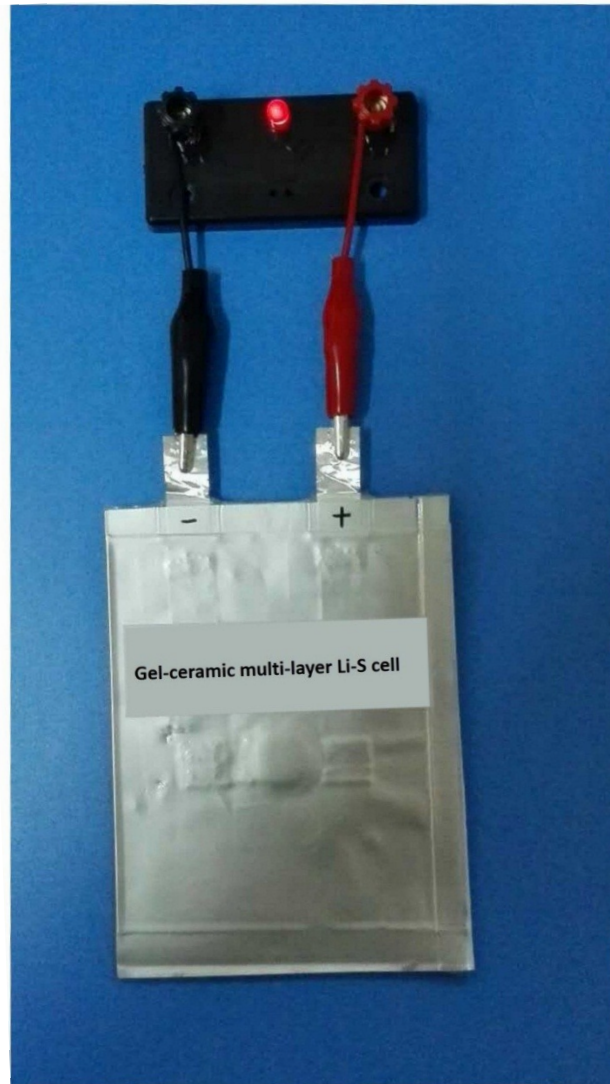
Fig. S1 An experimental demonstration of the gel-ceramic multi-layer Li-S cell.
