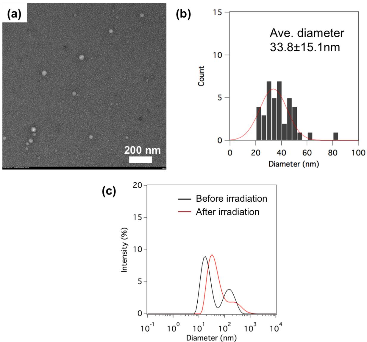
Fig. S2 (a) TEM image and (b) size distribution obtained from TEM images of Ls-CHP after 10 min photo irradiation. (c) size distribution of Ls-CHP nanogels in PBS buffer before and after photo irradiation.
