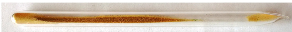
Compound 1 deposited on alumina after heating at 200 °C for 10 min
