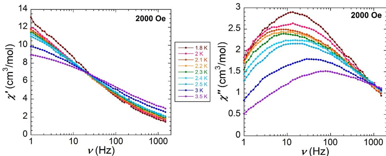
**Fig. S6:** In-phase (left) and out-of-phase susceptibility (right) of  $\text{Fe}_6\text{Dy}_3$  (**2**) under an applied field of 2000 Oe.
