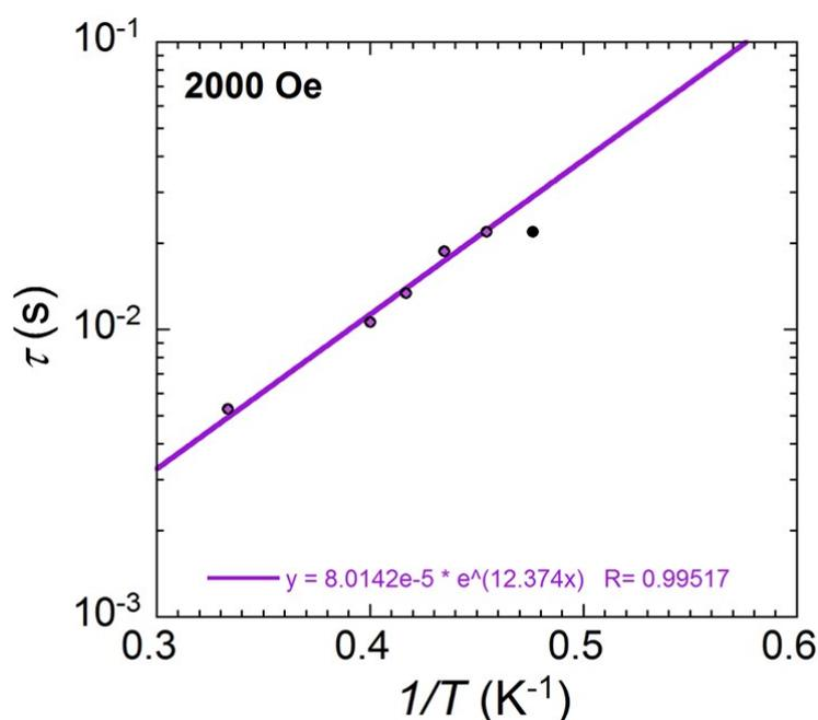
**Fig. S7:** Arrhenius fit for  $\text{Fe}_6\text{Dy}_3$  (**2**).
