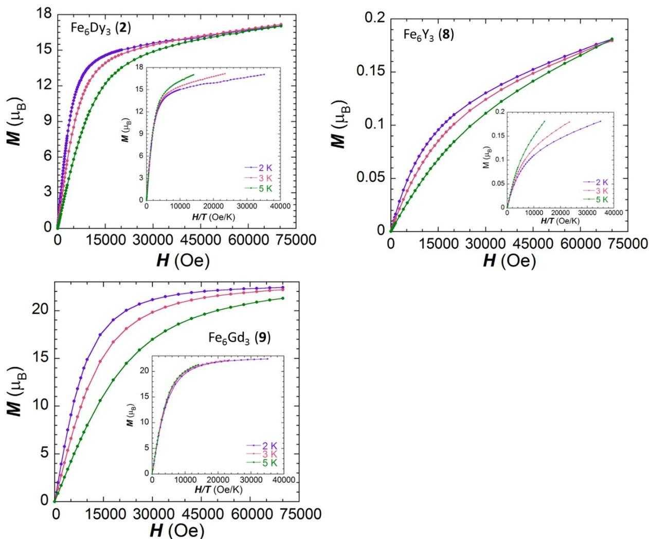
**Fig. S4:** Field dependence of Magnetization for Fe<sub>6</sub>Dy<sub>3</sub> (2) (left), Fe<sub>6</sub>Y<sub>3</sub> (8) (right) and Fe<sub>6</sub>Gd<sub>3</sub> (9) at different temperatures; reduced magnetization (inset).
