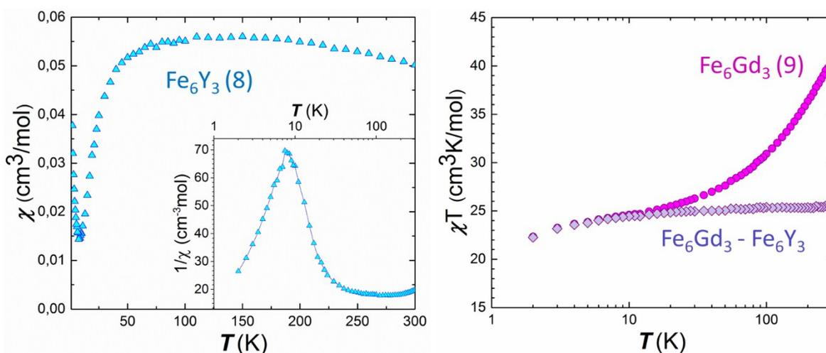
**Fig. S3:** Temperature dependence of the  $\chi$  plot at 1000 Oe for complexes  $\text{Fe}_6\text{Y}_3$  (**8**) (blue triangles) and the  $1/\chi$  plot with logarithmic x-axis (inset) (left) and  $\chi T$  plot of  $\text{Fe}_6\text{Gd}_3$  (**9**) and the substituted  $\chi T$  plot ( $\text{Fe}_6\text{Gd}_3 - \text{Fe}_6\text{Y}_3$ ) on a logarithmic temperature scale (right).
