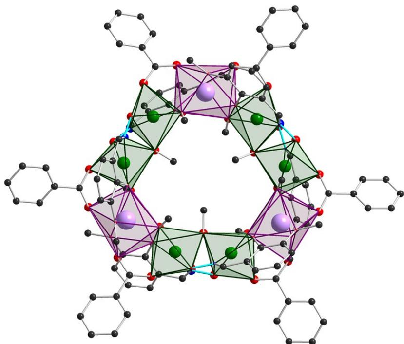
**Fig. S1:** Structure of Fe<sub>6</sub>Dy<sub>3</sub> (**2**) with polyhedra around the metal center to emphasize the distorted bicapped trigonal-prismatic geometry of the Ln<sup>III</sup> and the distorted octahedral environment of the Fe<sup>III</sup> ions.
