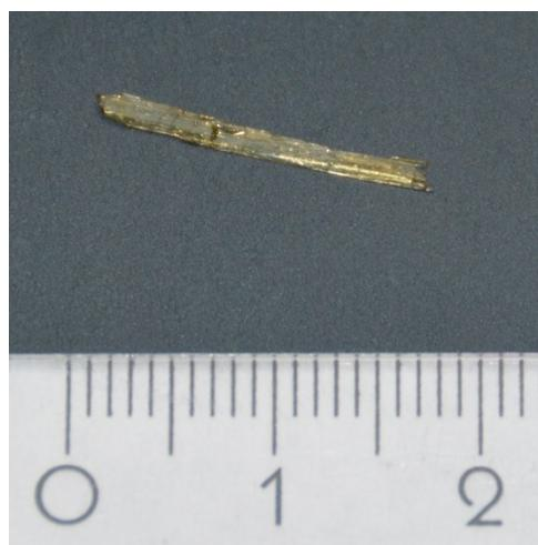
Fig. S1: Large *krypto-1* crystal obtained by very slow evaporation from a hexane solution: 1.75 cm and 13.01 mg
