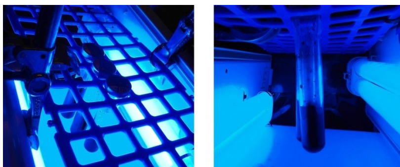
Figure S2: Irradiation setup 2. Blue CFL, 2 × 18 W / 2 × 2.73 cd / 450 ± 50 nm.
