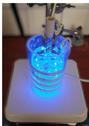
Figure S1: Irradiation setup 1. Blue LED, 5.4 W / 0.87 cd / 450 ± 25 nm.
