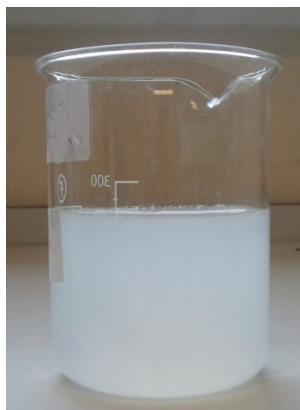
Fig. S4 Colloidal cellulose suspension in water prepared by ball-milling of microcrystalline \alpha -cellulose
