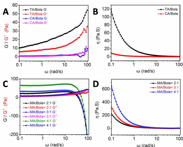
Figure S12: (A, C) Storage modulus  $G'$  and loss modulus  $G''$  versus frequency  $\omega$  (from 1 to 100 rad s<sup>-1</sup>), measured at 0.1% strain; (B, D) Complex viscosity determined by frequency  $\omega$ . (A, B) the molar ratio of TA (CA)/BolaHis is 4:1, (C, D) the molar ratio of MA/BolaHis is 2:1, 3:1, 4:1, respectively.
